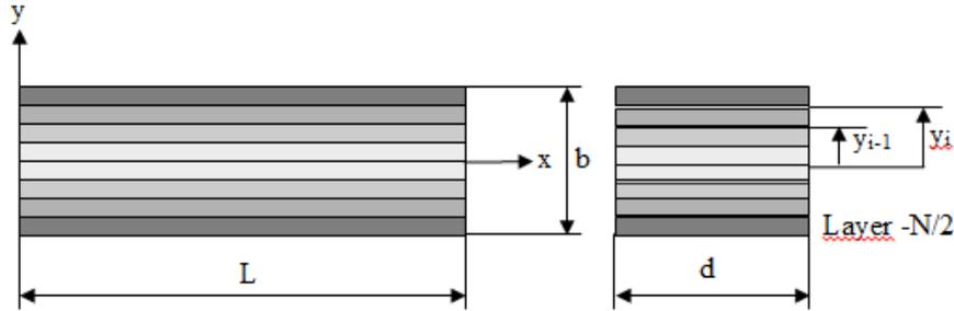
Fig. 1 Symmetric FGM sandwich beam
