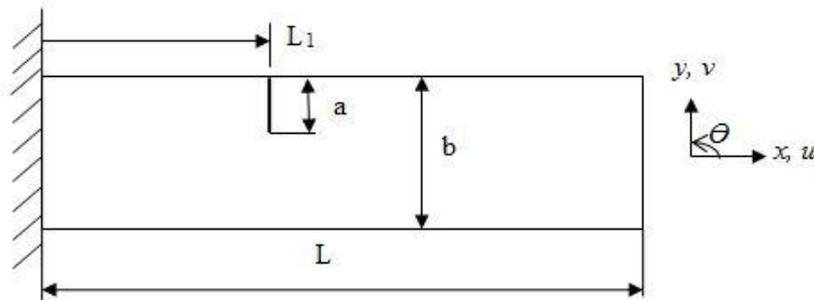
Fig. 2 Geometry of the cantilever isotropic homogeneous beam with an edge crack
