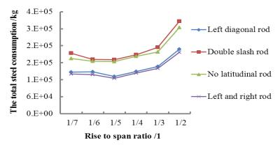
Fig. 16 The total steel consumption of four typical Schwedler spherical reticulated shells when span is 70 m
