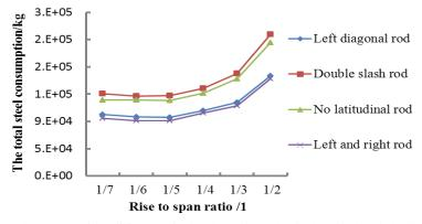
Fig. 15 The total steel consumption of four typical Schwedler spherical reticulated shells when span is 60 m
