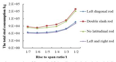
Fig. 14 The total steel consumption of four typical Schwedler spherical reticulated shells when span is 50 m
