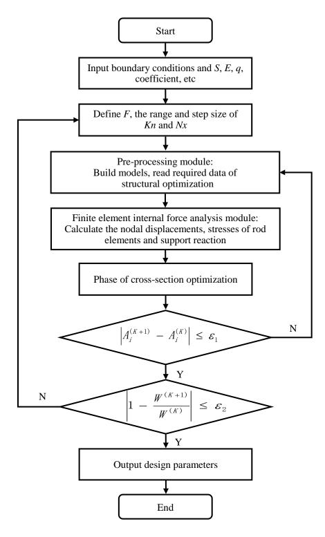
Fig. 11 Shape optimization flowchart of Schwedler spherical reticulated shells
