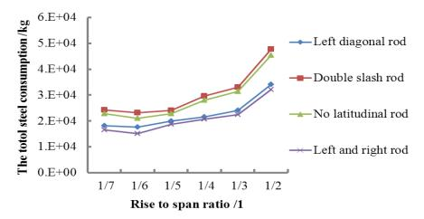
Fig. 12 The total steel consumption of four typical Schwedler spherical reticulated shells when span is 30 m
