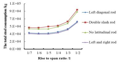
Fig. 13 The total steel consumption of four typical Schwedler spherical reticulated shells when span is 40 m
