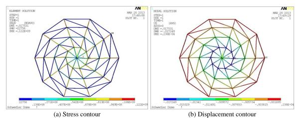
Fig. 10 Left diagonal rod - Schwedler spherical reticulated shell (S=30, F=6, Kn=10, Nx=4)
