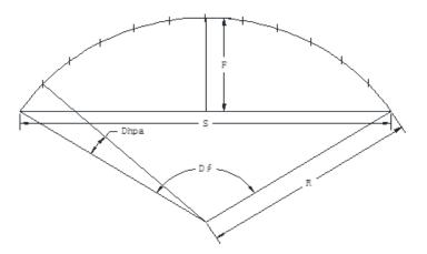
Fig. 2 Geometric schematic diagram of spherical reticulated shells
