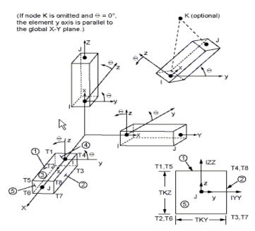
Fig. 9 Schematic diagram of Beam4 element (captured from ANSYS software documentation)
