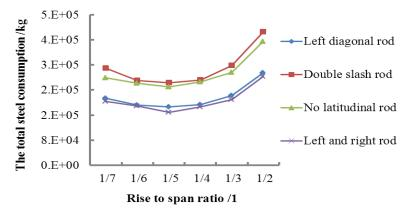
Fig. 17 The total steel consumption of four typical Schwedler spherical reticulated shells when span is 80 m
