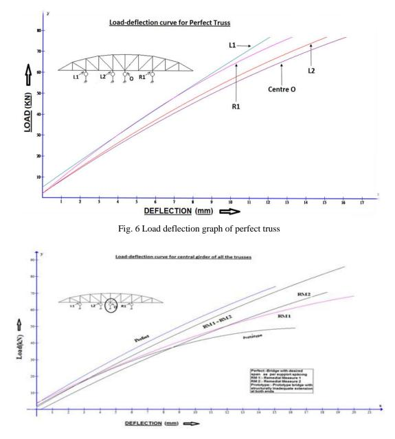
Fig. 7 Load deflection curve of 5 models at central location, O
