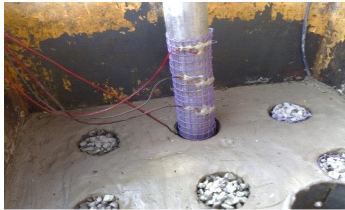
Fig. 9 Process of construction of encased stone columns
