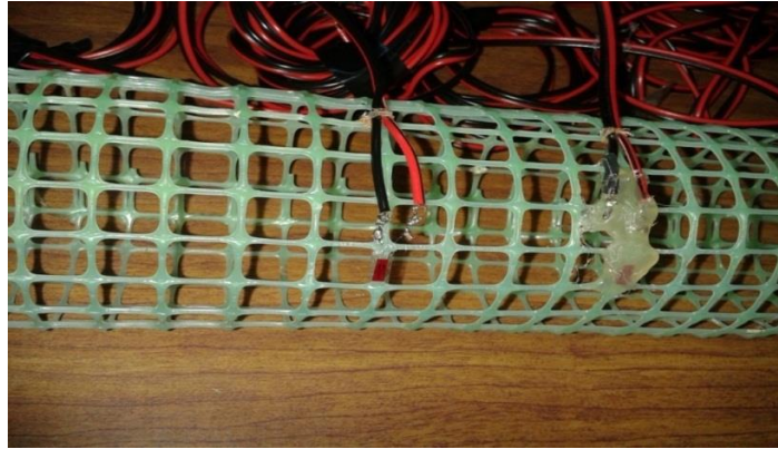
Fig. 8 Strain gauge fixed on geogrid
