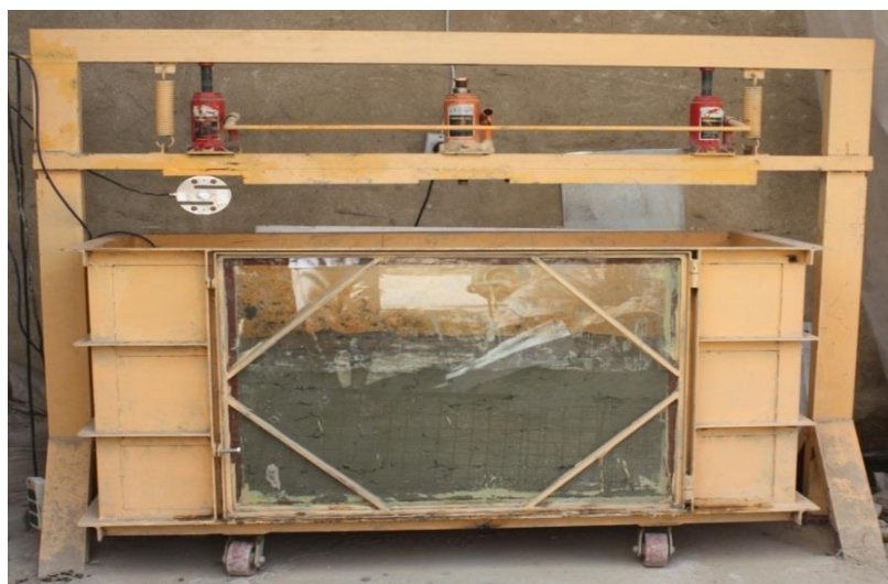
Fig. 4 Experimental test container and loading system
