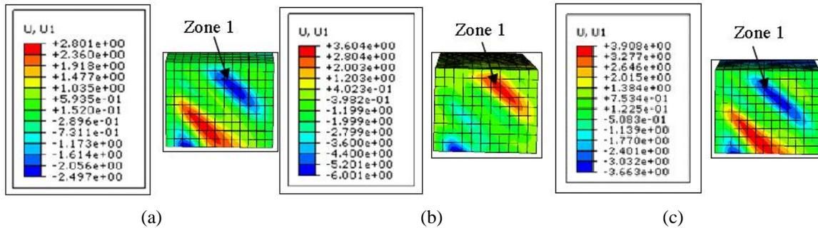
Fig. 15 Out-of-plane displacements for model M1 ( $B=20$  m,  $h=4$  m), in cm, (a)  $\delta_v=5$  mm, (b)  $\delta_v=9$  mm, (c)  $\delta_v=10$  mm
