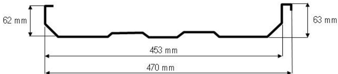
Fig. 4 Panel type U45. Cross Section
