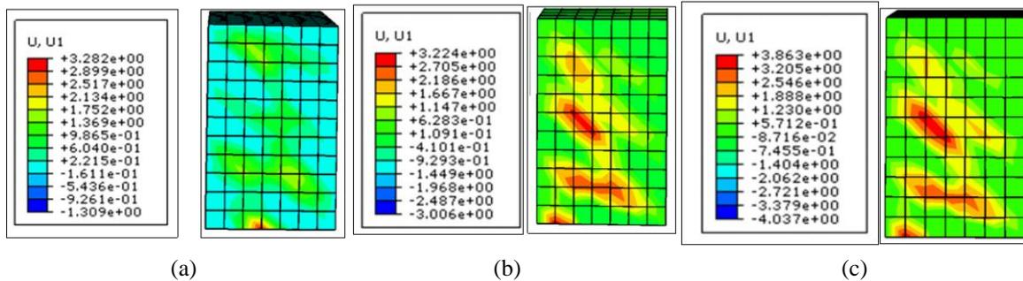
Fig. 19 Out-of-plane displacements for model M5 ( $B=20$  m,  $h=8$  m), in cm, (a)  $\delta_v=5$  mm, (b)  $\delta_v=7$  mm, (c)  $\delta_v=10$  mm
