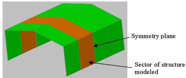
Fig. 8 Part of storehouse considered in computational model
