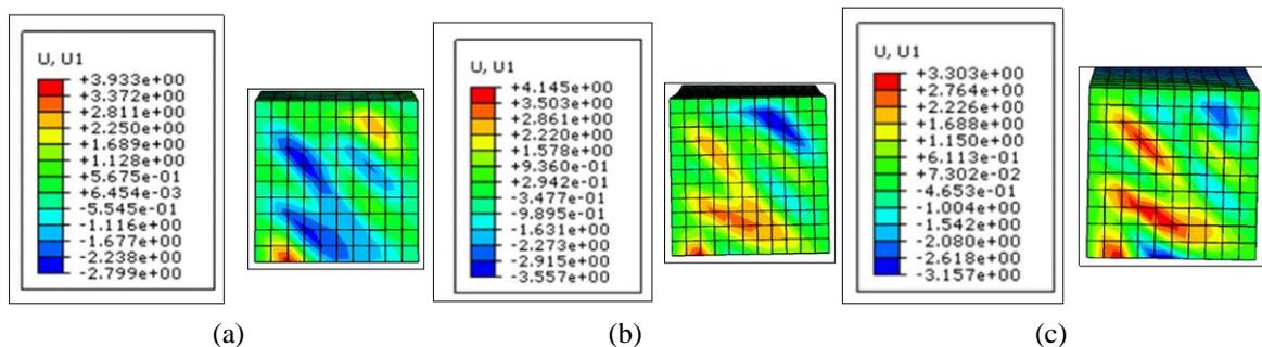
Fig. 16 Out-of-plane displacements for model M2 ( $B=20$  m,  $h=5$  m), in cm, (a)  $\delta_v=7$  mm, (b)  $\delta_v=9$  mm, (c)  $\delta_v=10$  mm
