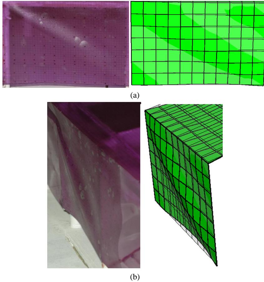
Fig. 12 Comparison between physical and computational models, (a) Front view, (b) Lateral view
