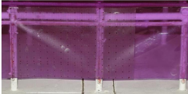
Fig. 7 Front view of the deformation in physical model due to differential settlement of central column ( $\delta_{vmax}=2$  mm)
