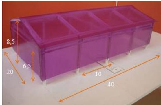
Fig. 5 Small-scale physical model, dimensions in cm
