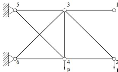
Fig. 3 Unfeasible topology due to necessary condition 2
