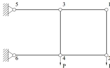
Fig. 4 Unfeasible topology due to necessary condition 3
