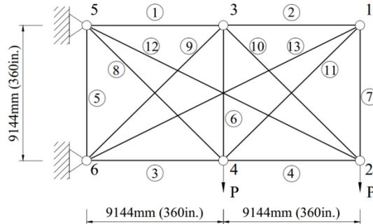
Fig. 7 13-bar truss ground structure
