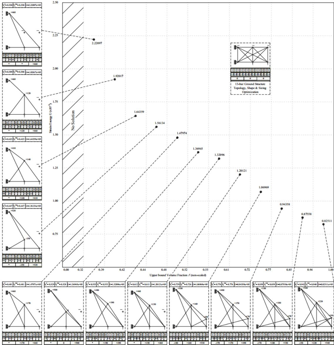
Fig. 11 Solutions for topology, shape & sizing optimization for 13-bar truss ground structure
