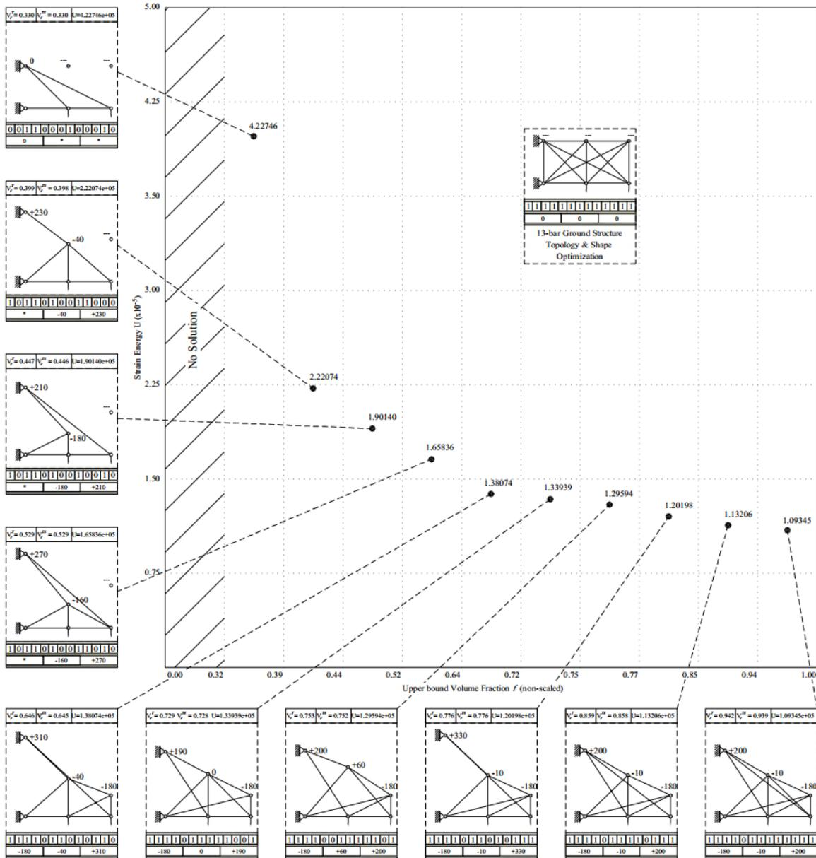
Fig. 10 Solutions for topology & shape optimization for 13-bar truss ground structure
