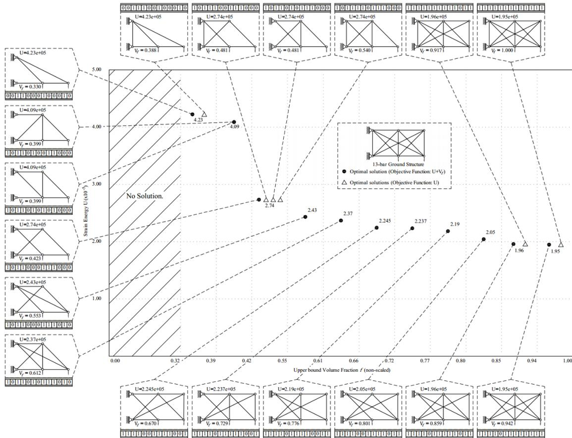
Fig. 8 Solutions for pure topology optimization for 13-bar truss ground structure
