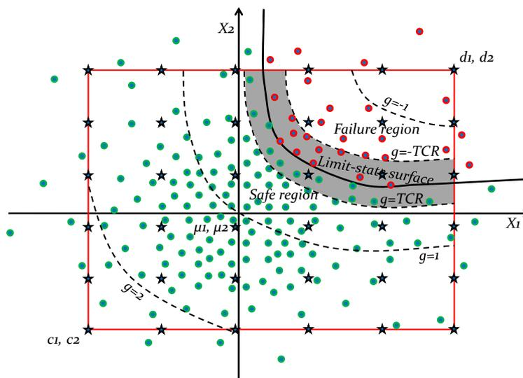
Fig. 4 Details of concepts of the proposed method for non-truncated random variables
