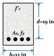
Fig. 7 Cross section of RC beam
