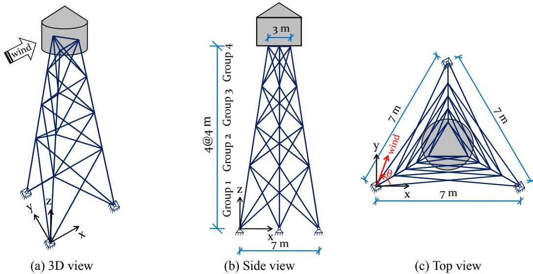
Fig. 10 Three-dimensional 39-bar truss
