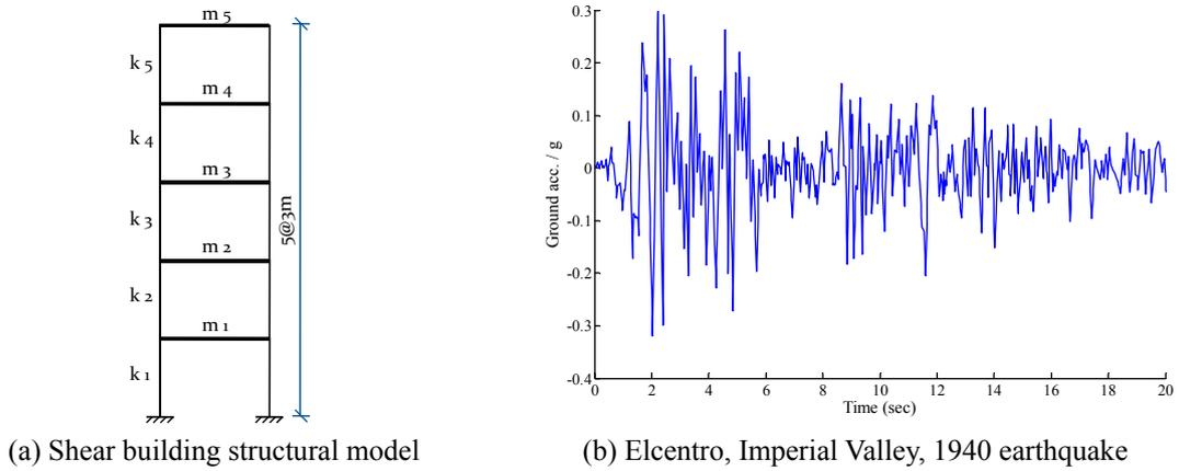
Fig. 9 Seismically excited building
