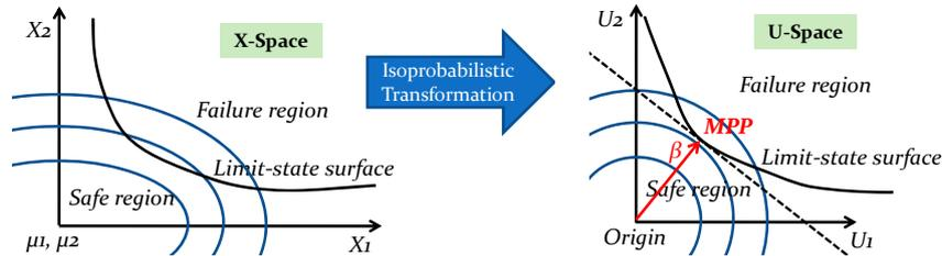
Fig. 1 Isoprobabilistic transformation and reliability measures
