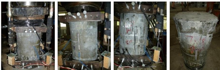
Fig. 6 Specimen loading and failure state
