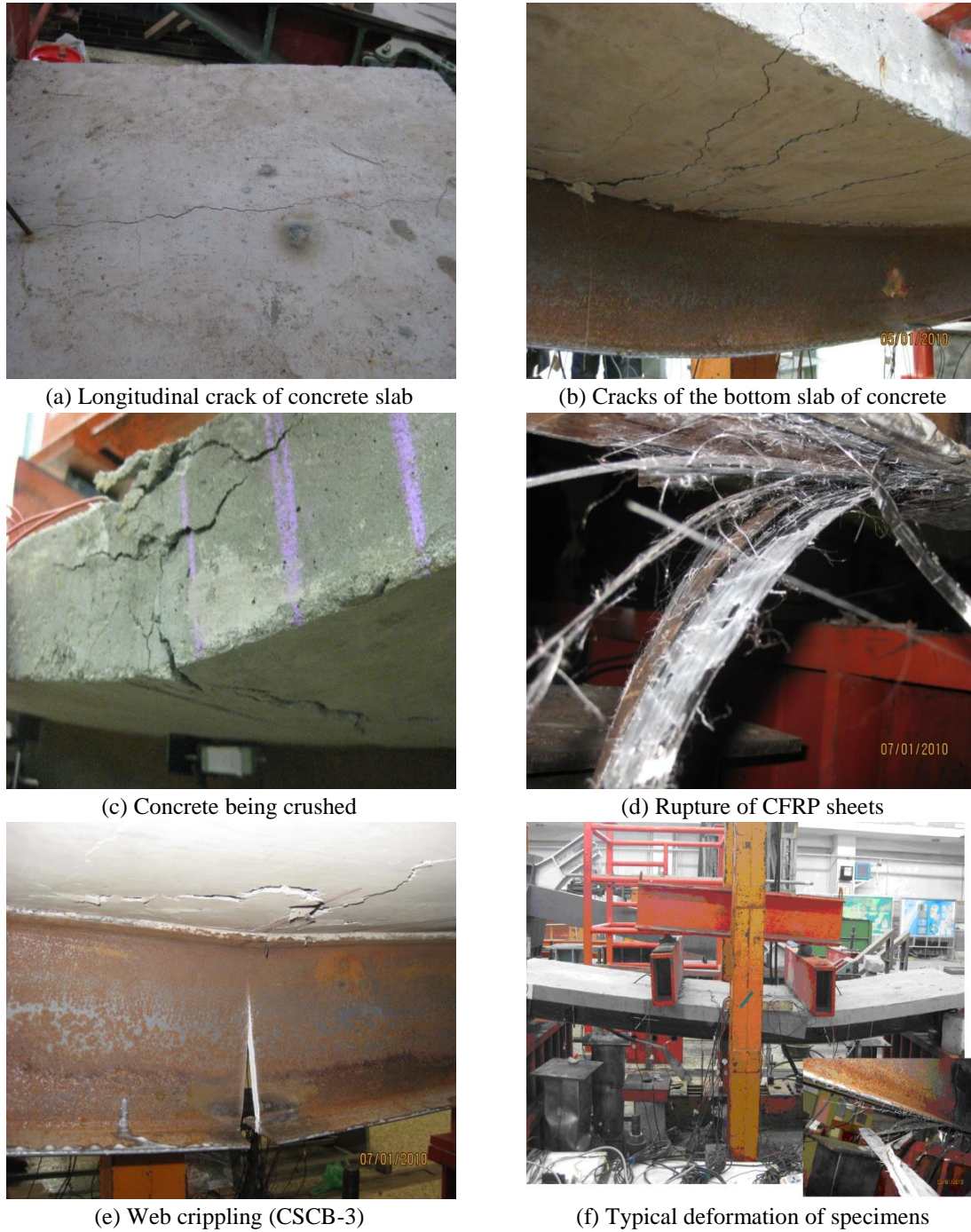
Fig. 4 Failure modes of test specimens
