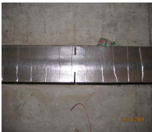
(a) Corroded model
