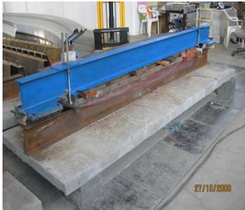
(e) Paste prestressed CFRP sheets
