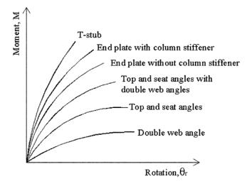
Fig. 2 Moment-rotation curves of semi-rigid connections
