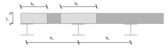
Fig. 4 Effective width of composite beam
