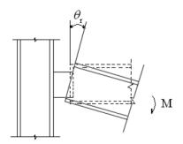
Fig. 1 Rotation of a semi-rigid connection
