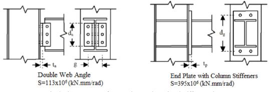
Fig. 3 The two types of connections and rotational stiffness values
