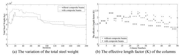
Fig. 12 Semi rigid steel frame with End Plate with Column Stiffness connection with and without composite beams
