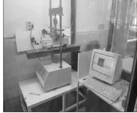
Fig. 5 The four-point flexural test put forward in ASTM C1018 (the textile layer is shown in red color)
