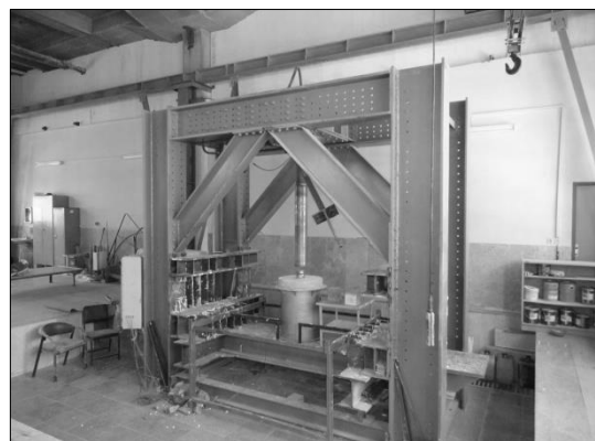
Fig. 14 The testing setup of slabs.
