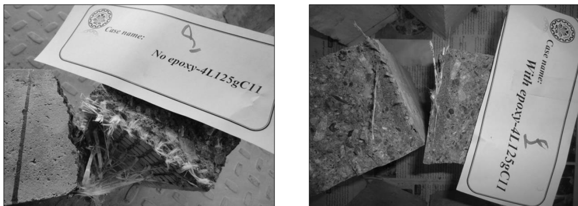
Fig. 11 Comparison between the fracture patterns belonging to E5L125gC11 (with the intermediate layer) and 5L125gC11 (without the intermediate layer)
