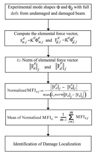
Fig. 1 Damage identification algorithm based on modal force index
