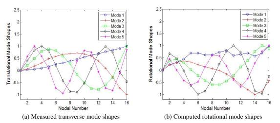
Fig. 4 Measured transverse mode shapes and computed rotational mode shapes for the undamaged case
