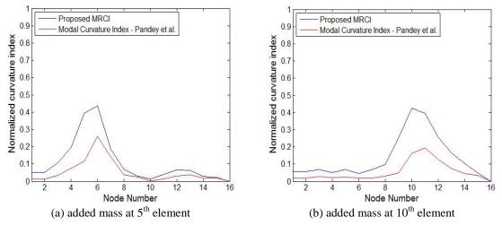
Fig. 7 The experimental results of mean of normalized MRCI and MCI proposed by Pandey *et al.* for the cases of the added mass at  $5^{th}$  and at  $10^{th}$  element individually.
