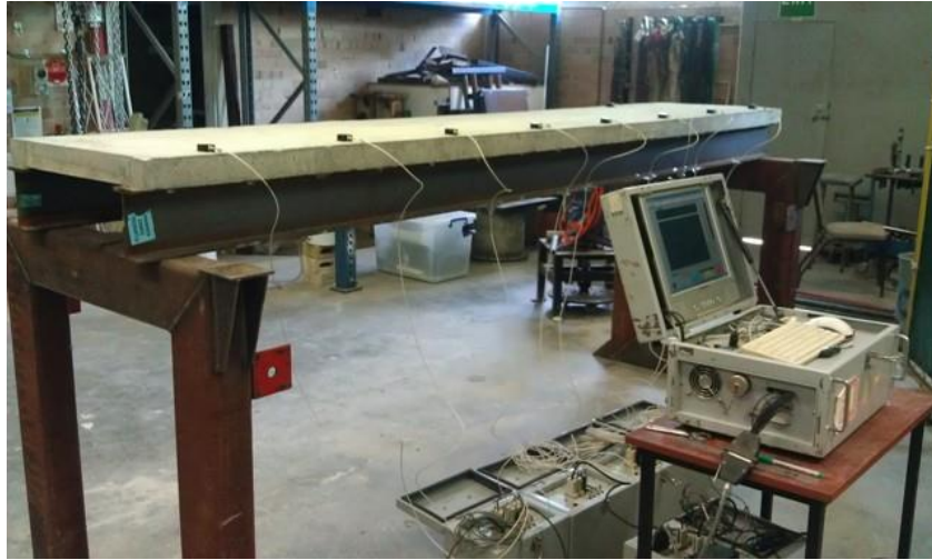
Fig. 11 Experimental setup of the slab-on-girder structure
