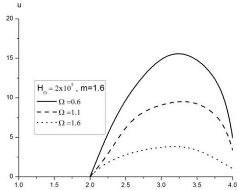
Fig. 4 Variation of the radial displacement with the radial, when magnetic field  $H_0=2 \times 10^3$ , the non-homogeneity  $m=1.6$  at different values for rotation  $\Omega=0.6, 1.1, 1.6$ , in case I
