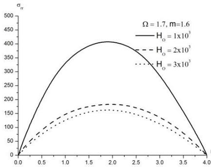
Fig. 11 Variation of the radial component of the stress  $\sigma_{rr}$  with the radial  $r$ , when rotation  $\Omega=0.6$ , the non-homogeneity  $m=1.6$  at different values for magnetic field  $H_0$ , in case II
