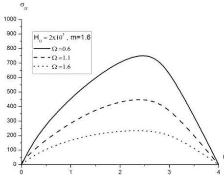
Fig. 5 Variation of the radial stress with the radial, when magnetic field  $H_0=2\times 10^3$ , the non-homogeneity  $m=1.6$  at different values for rotation  $\Omega=0.6, 1.1, 1.6$ , in case I
