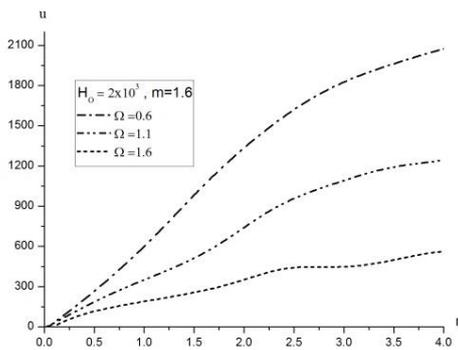
Fig. 13 Variation of the radial displacement with the radial, when magnetic field  $H_0=2\times 10^3$ , the non-homogeneity  $m=1.6$  at different values for rotation  $\Omega=0.6, 1.1, 1.6$ , in case II
