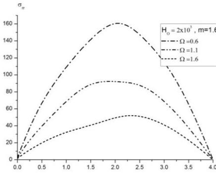
Fig. 14 Variation of the radial stress with the radial, when magnetic field  $H_0=2\times 10^3$ , the non-homogeneity  $m=1.6$  at different values for rotation  $\Omega=0.6, 1.1, 1.6$ , in case II
