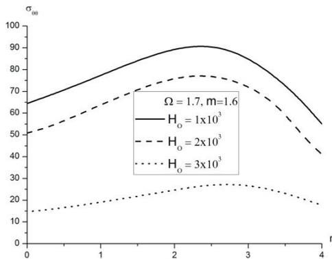
Fig. 3 Variation of the tangential component of the stress  $\sigma_{\theta\theta}$  with the radial  $r$ , when rotation  $\Omega=0.6$ , the non-homogeneity  $m=1.6$  at different values for magnetic field  $H_0$ , in case I
