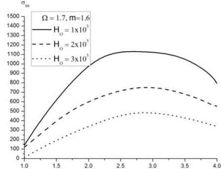
Fig. 12 Variation of the tangential component of the stress  $\sigma_{\theta\theta}$  with the radial  $r$ , when rotation  $\Omega=0.6$ , the non-homogeneity  $m=1.6$  at different values for magnetic field  $H_0$ , in case II
