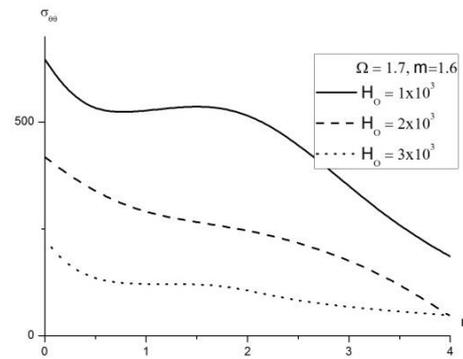
Fig. 6 Variation of the tangential stress with the radial, when magnetic field  $H_0=2\times 10^3$ , the non-homogeneity  $m=1.6$  at different values for rotation  $\Omega=0.6, 1.1, 1.6$ , in case I
