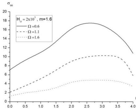
Fig. 15 Variation of the tangential stress with the radial, when magnetic field  $H_0=2\times 10^3$ , the non-homogeneity  $m=1.6$  at different values for rotation  $\Omega=0.6, 1.1, 1.6$ , in case I
