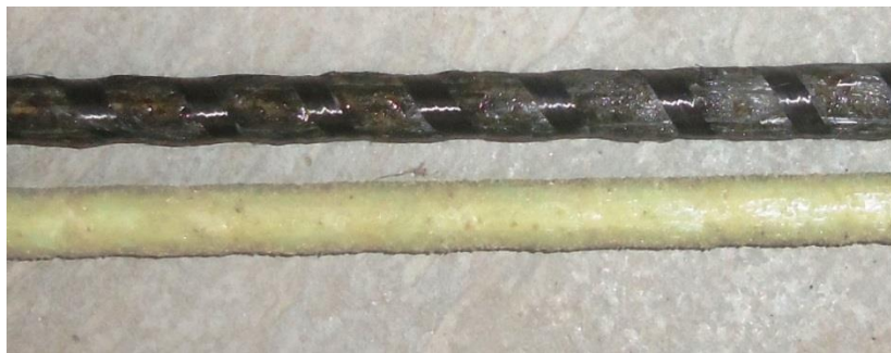
Fig. 2 Reinforcing bars: CFRP (top) and GFRP (bottom)
