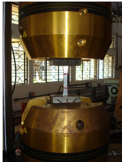
(a) Tension test set-up on aluminium alloy specimen
