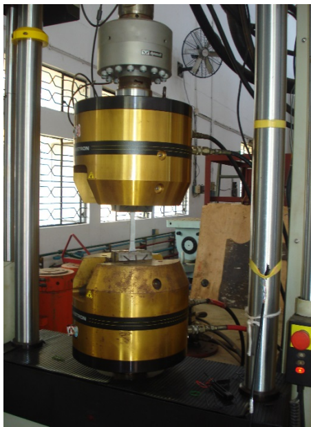
(a) Tension test set-up on aluminium alloy specimen
