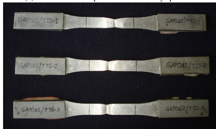
(b) Tension test specimens after failure
