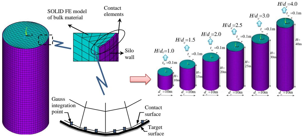
Fig. 1 Finite element model for silos and schematic view for their dimensions (Durmuş 2013)
