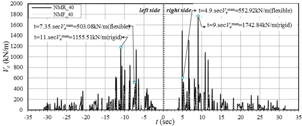
Fig. 8 Variations of equivalent base shears with time at opposed sides of the silo wall for for slenderness ratio of 4.0 via NMR and NMF
