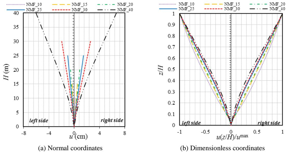
Fig. 4 Comparison of the maximum horizontal displacements along the height of the silo wall via NMF
