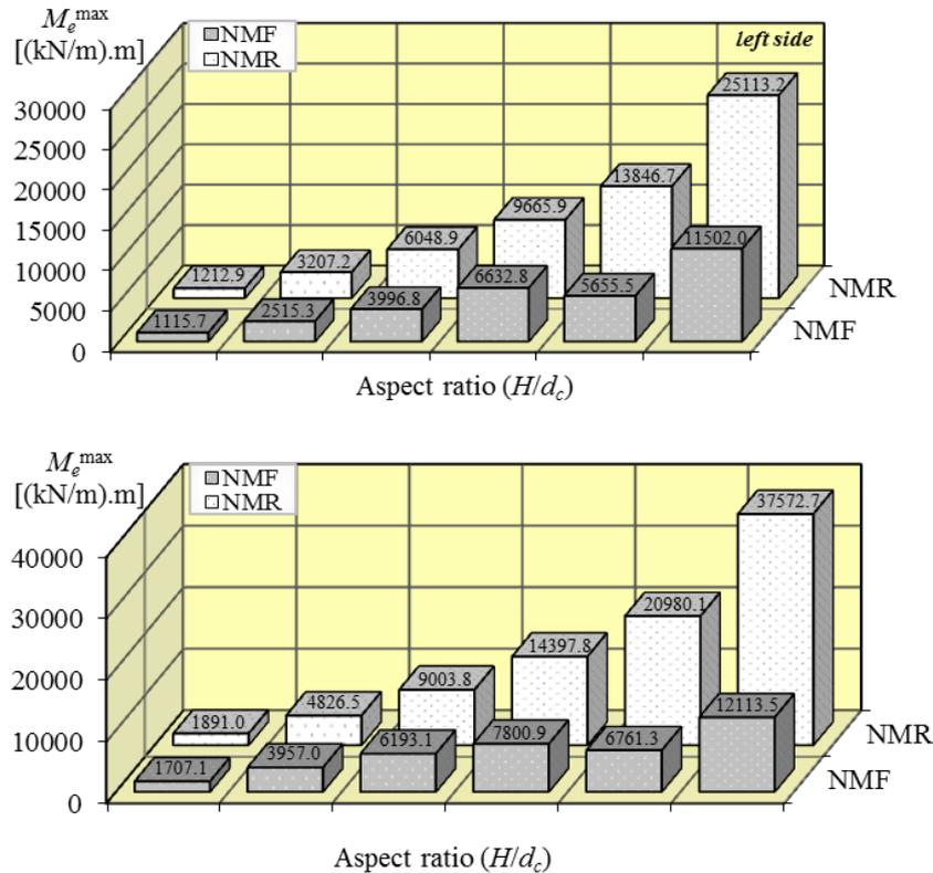
Fig. 9 Maximum equivalent overturning moment variations with increasing slenderness ratio via NMF and NMR
