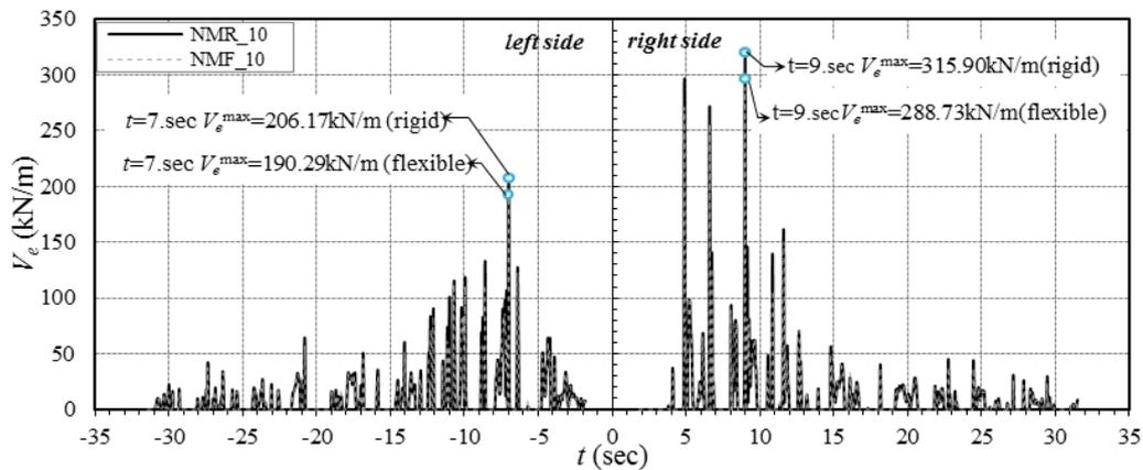
Fig. 6 Variations of equivalent base shears with time at opposed sides of the silo wall for slenderness ratio of 1.0 via NMR and NMF
