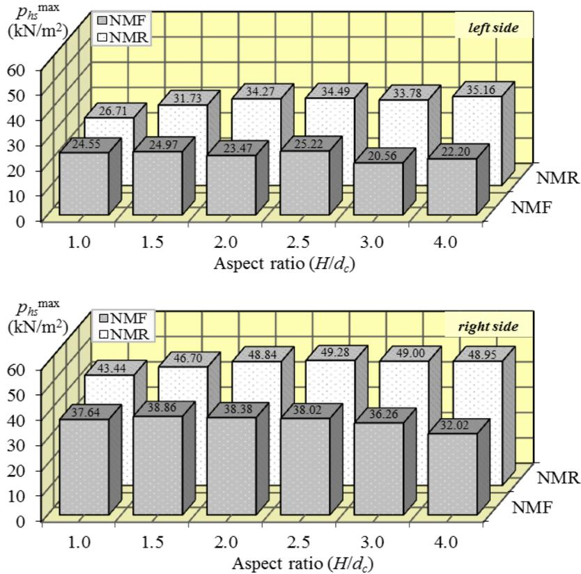
Fig. 2 Maximum dynamic material pressure variations with increasing slenderness ratio via NMF and NMR
