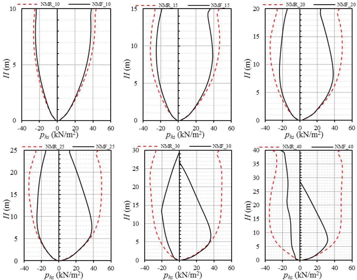
Fig. 3 Comparison of the dynamic material pressures along the height of the silo wall for six different slenderness ratios according to NMR and NMF
