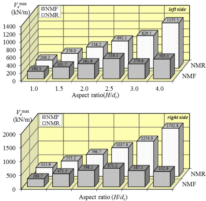
Fig. 5 Maximum equivalent base shear force variations with increasing slenderness ratio via NMF and NMR
