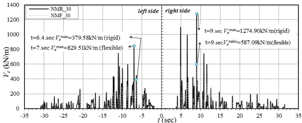
Fig. 7 Variations of equivalent base shears with time at opposed sides of the silo wall for slenderness ratio of 3.0 via NMR and NMF
