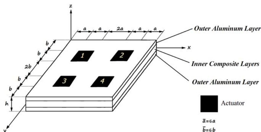
Fig. 1 A FML panel with distributed piezoelectric actuators
