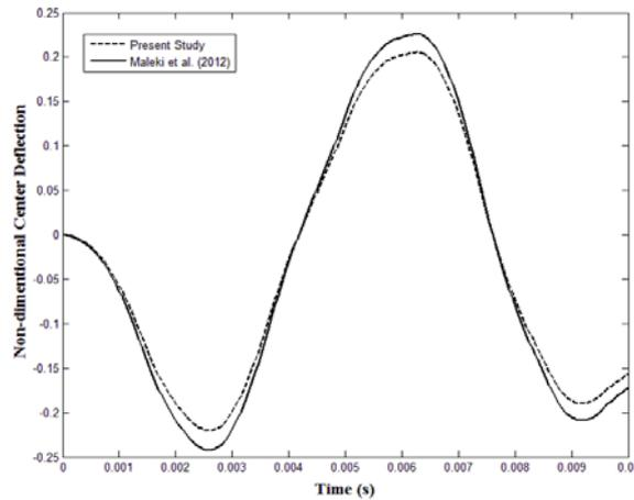
Fig. 4 Response of orthotropic, square, clamped panel to conventional blast load
