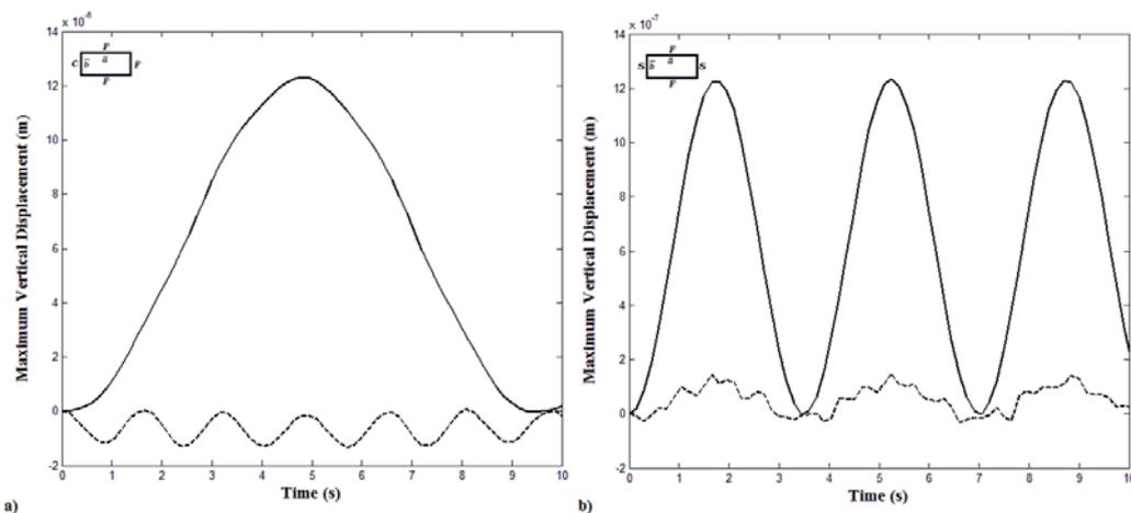
Fig. 7 Optimum solutions of symmetric 8-layered FML panels obtained by E-ABC algorithm for different boundary conditions and  $[Al/45/-45/45]_s$  stacking sequence ( $\bar{a}/\bar{b}=1$ ): (a) CFFF, (b) SFSE, (c) SSSS, (d) CSCS, (e) CCFF, (f) CCCC; —Non-optimized response, ---Optimized response
