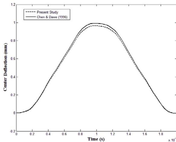
Fig. 3 Response of isotropic, square, simply supported panel to uniformly distributed step load
