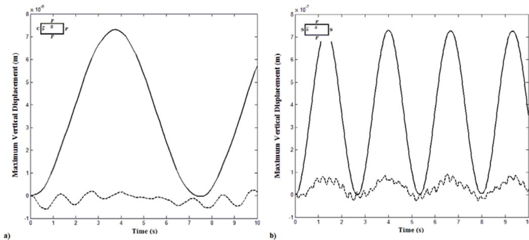
Fig. 5 Optimum solutions of symmetric 8-layered FML panels obtained by E-ABC algorithm for different boundary conditions and [Al/0/0/0]<sub>s</sub> stacking sequence ( $\bar{a}/\bar{b} = 1$ ) : (a) CFFF, (b) SFSF, (c) SSSS, (d) CSCS, (e) CCFF, (f) CCCC;—Non-optimized response, ---Optimized response
