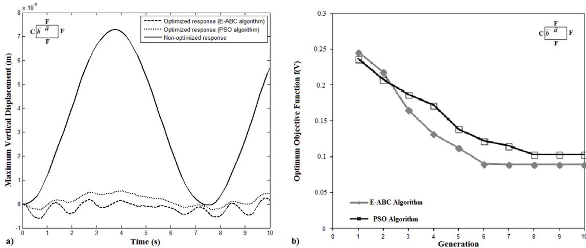
Fig. 2 Comparison of the E-ABC and PSO results for CFFF edge condition for symmetrically FML 8-layered square panel with the same generations
