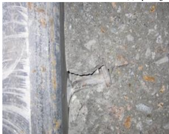
(c) Excessive deformation of a stud connector
