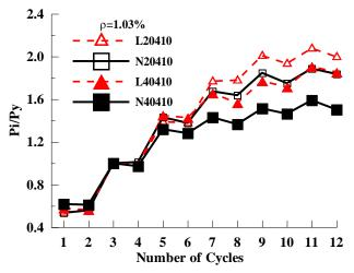
Fig. 9 Effect of concrete strength on the degradation of the flexural strength of beam
