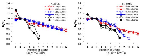
Fig. 12 Effect of tension reinforcement on the stiffness degradation of beam
