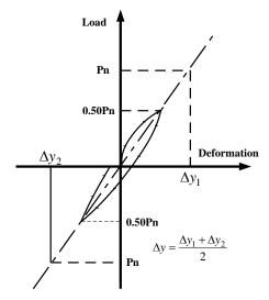
Fig. 3 Determination of yielding displacement  $\Delta y$
