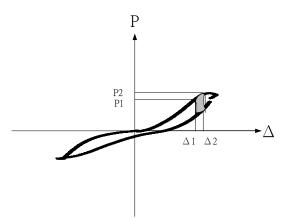
Fig. 13 Calculation of the energy dissipation capacity
