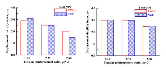
Fig. 7 Displacement ductility index versus tension reinforcement ratio
