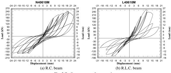
Fig. 5 Cyclic responses of concrete beam
