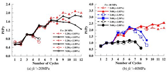
Fig. 11 Effect of tension reinforcement on the degradation of the flexural strength of beam
