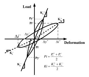
Fig. 8 Definitions of strength and stiffness
