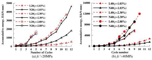
Fig. 16 Effect of tension reinforcement on the energy dissipation of beam
