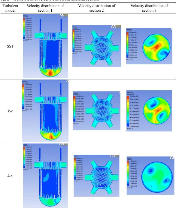
Table 4 Comparison of velocity contours at different sections
