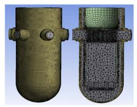
Fig. 4 Mesh of hydrodynamic analysis model including structural region
