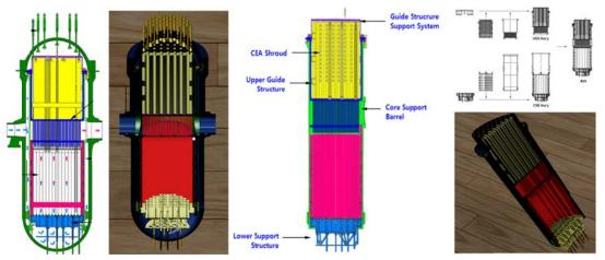
Fig. 1 Schematics and VR snapshots for reactor internals of OPR1000
