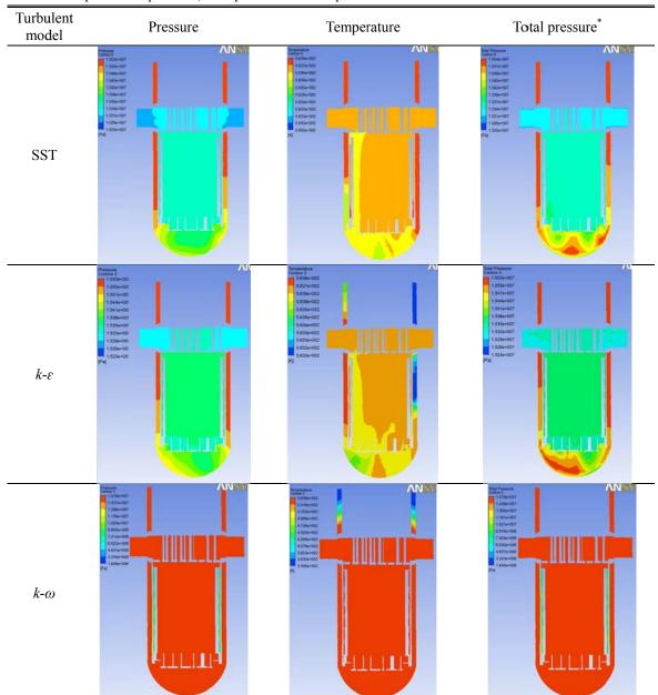
Table 5 Comparison of pressure, total pressure and temperature contours at section 1
