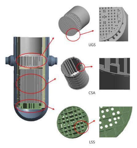
Fig. 3 Integrated CAD model of reactor internals used in the present study
