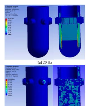
(b) 480 Hz Fig. 6 Acoustic pressures distributions obtained from periodic hydrodynamic analyses
