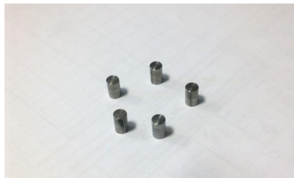
Fig. 3 Hot compression test specimens before testing
