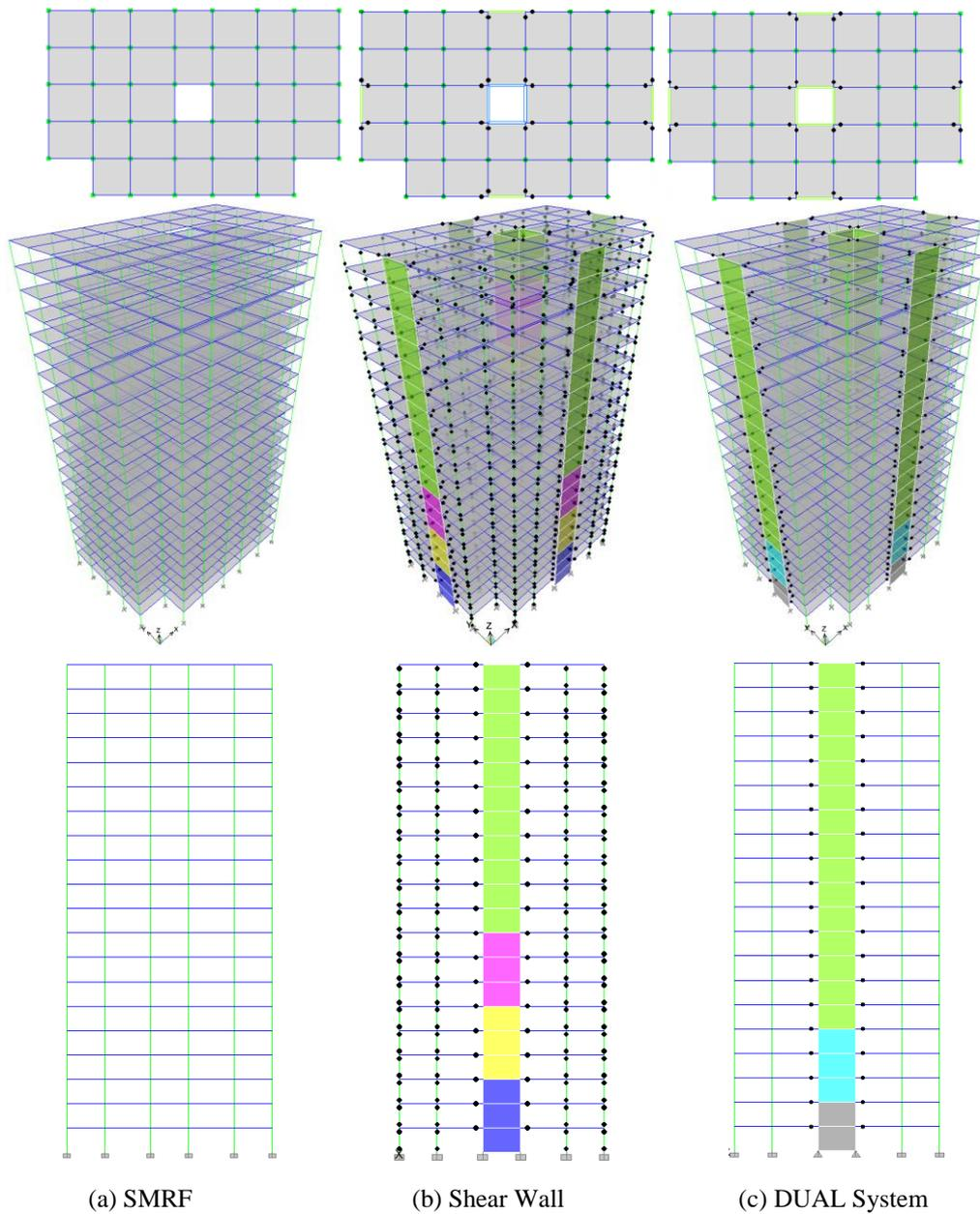
Fig. 2 20 Story Plan, 3D View and Elevation
