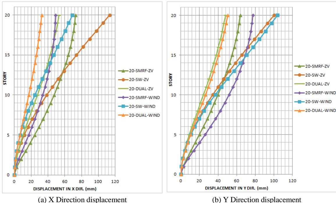
Fig. 6 20-Story Vs displacement due to Seismic & Wind force
