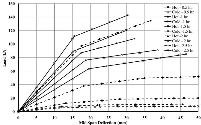
Fig. 18 Comparison of load deflection in 'Hot' and 'Cold' conditions
