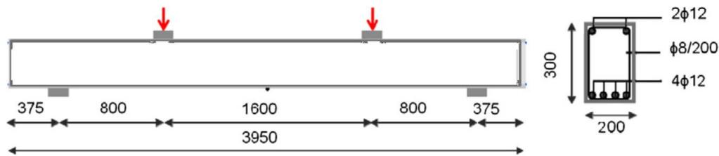
Fig. 12 Test setup for strength test on RC beams (Ozbolt *et al.* 2013)
