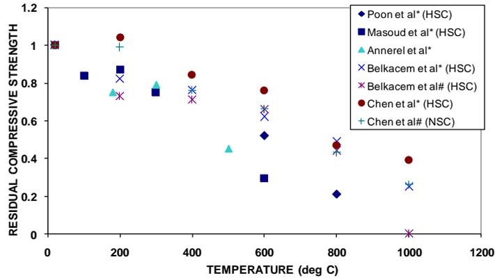
Fig. 4 Variation of residual compressive strength with temperature for concrete (Residual) (\*- Air cooled, #- Water cooled)
