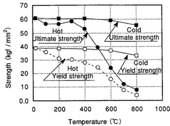
Fig. 5 Variation of Yield and ultimate strength of reinforcing bars as a function of temperature (Takeuchi *et al.* 1993)
