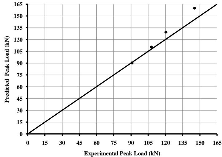
Fig. 15 Experimental v/s predicted Peak load comparison
