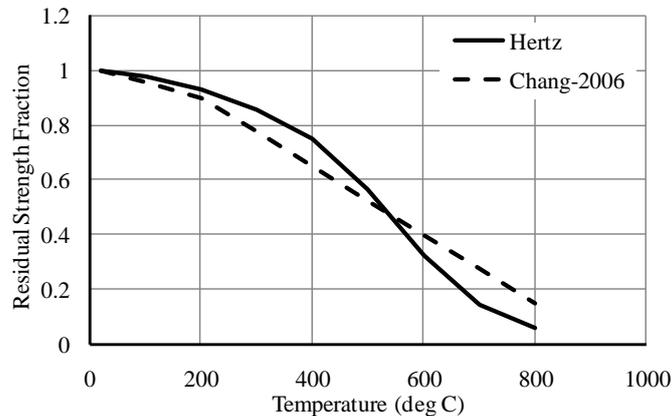
Fig. 8 Comparison of Hertz (2005) model with cold condition experimental results of Chang *et al.* (2006)
