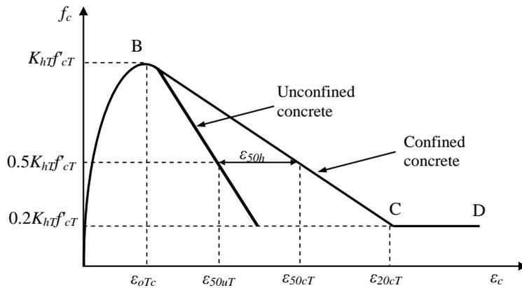
Fig. 7 Stress strain curve for concrete in compression (Youssef and Moftah 2007)
