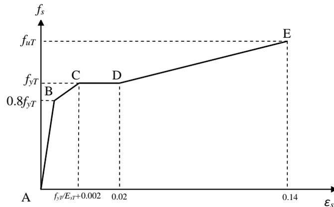
Fig. 9 Idealized stress-strain curve of reinforcing bars in tension or compression
