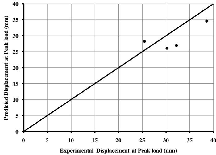
Fig. 17 Experimental v/s predicted deflections at peak load
