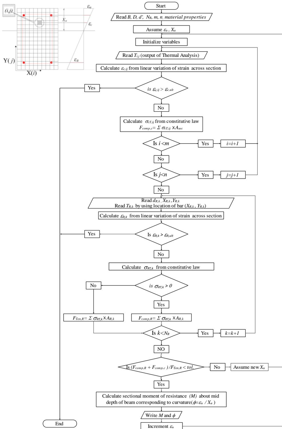
Fig. 10 Flowchart for moment-curvature analysis for the section
