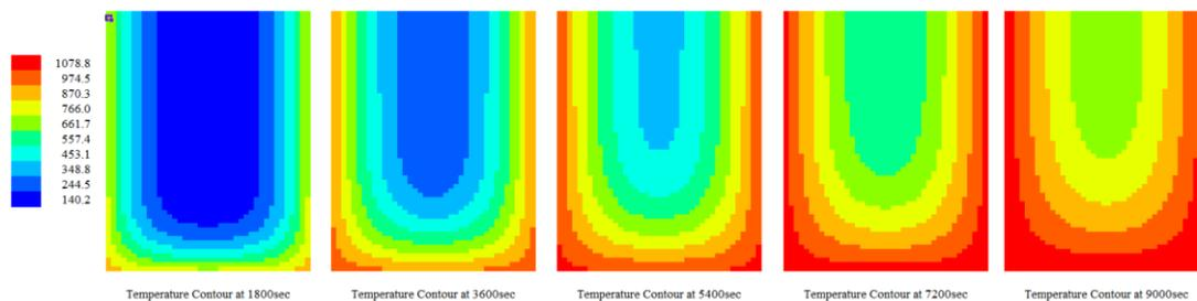
Fig. 13 Temperature contour across beam cross section at 0.5 h, 1.0 h, 1.5 h, 2.0 h and 2.5 h
