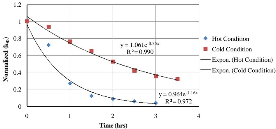
Fig. 11 Normalized stiffness degradation due to fire exposure (Hot and cold conditions)
