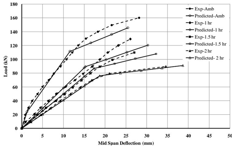
Fig. 14 Comparison of predicted load deflections with experimental values
