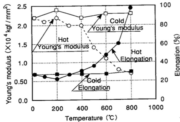
Fig. 6 Variation of Young's modulus and elongation of reinforcing bars with temperature (Takeuchi *et al.* 1993)
