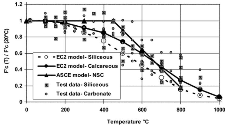
Fig. 3 Variation of compressive strength with temperature for normal strength concrete (Hot condition) (Kodur *et al.* 2008)
