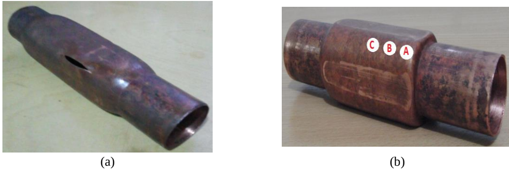
Fig. 9 (a) The ruptured tube in initial bulge phase because of improper pressure in 17 MPa pressure, (b) the formed tube by using P_3 pressure profile
