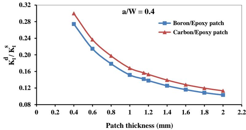
Fig. 5 Effect of patch thickness on the SIF (single and double sided repair)
