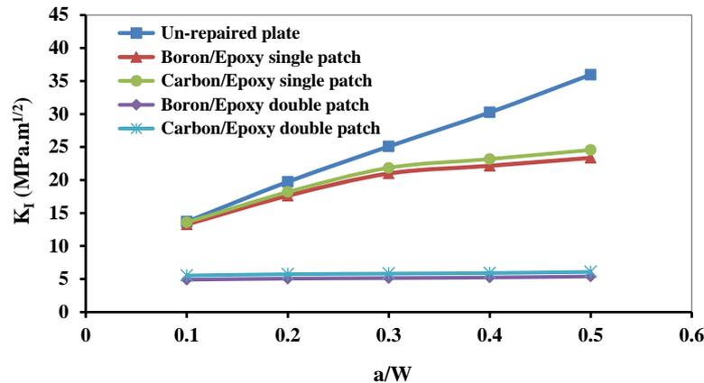
Fig. 4 Variation of  $K_I$  versus crack length for single and double patched and un-patched centre cracked plate
