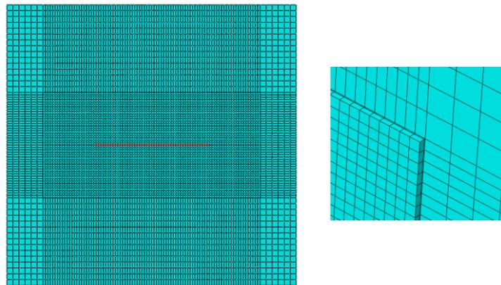
Fig. 3 The mesh of repaired cracked plate using XFEM
