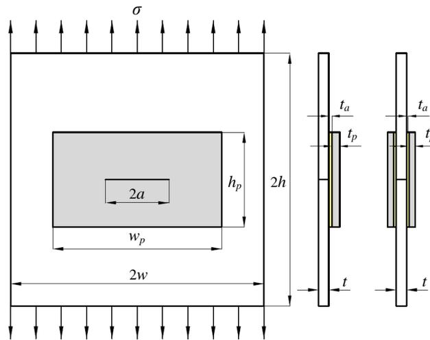
Fig. 2 Geometrical model of the centre cracked plate with single and double patch under pure mode I
