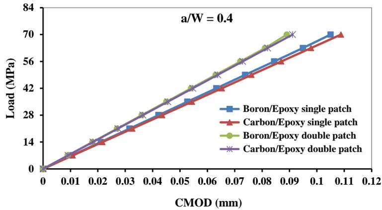
Fig. 9 Effect of single and double symmetric repairing patches on the CMOD
