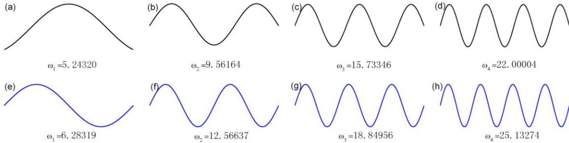
Fig. 2 First eight in-plane mode shapes and natural frequencies of the suspended cable: (a)-(d) the first four symmetric mode shapes and natural frequencies; (e)-(h) the first four anti-symmetric mode shapes and natural frequencies
