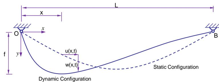
Fig. 1 Two different configurations of the suspended cable
