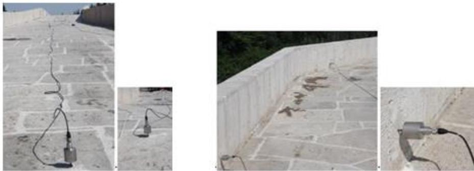
Fig. 12 The accelerometer connections on Aspendos Masonry Arch Bridge
