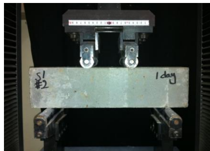
Fig. 2 4-point loading flexural test (ASTM C 1609); (a) geometry of specimen, (b) test setup
