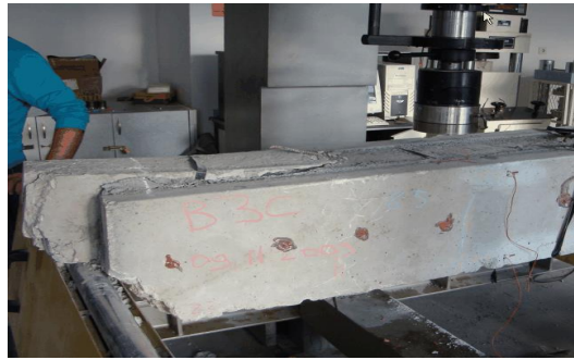
Fig. 14 Failure of strengthened beam
