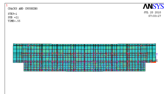
Fig. 17 Cracks of B1c1 beam at failure
