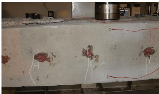
Fig. 17 Cracks of B1c1 beam at failure
