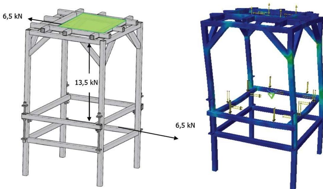
Fig. 12 Loads applied to SPIF-A’s frame and subsequent (scaled for visibility) deflection
