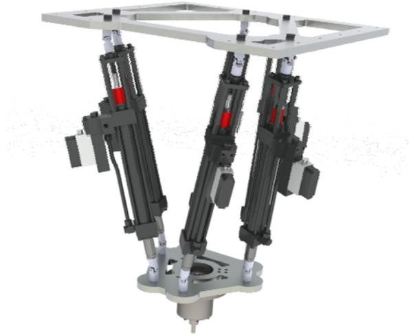
Fig. 10 Kinematic system for SPIF-A composed of Stewart platform and spindle
