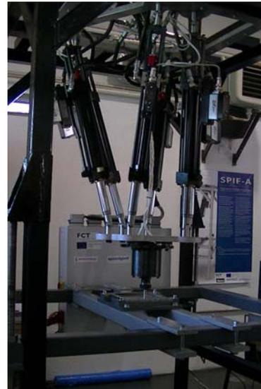
Fig. 14 Prototype of SPIF-A. (a) CAD model; (b) built Machine
