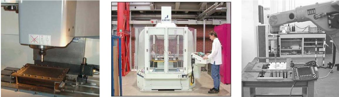
Fig. 1 Equipment for performing ISF. From left to right: adapted milling machine (Ambrogio *et al.* 2005, Amino purpose built machine, and serial manipulator (Strano 2005)
