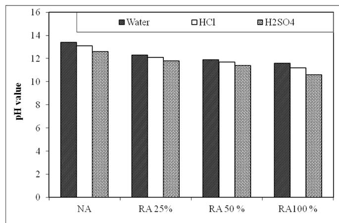
Fig. 7 Alkalinity of concrete specimens
