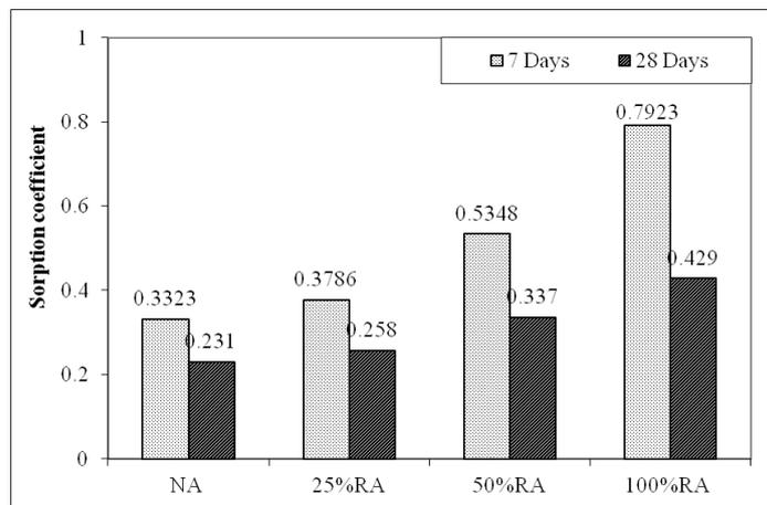
Fig. 5 Effect of RA on sorption coefficient
