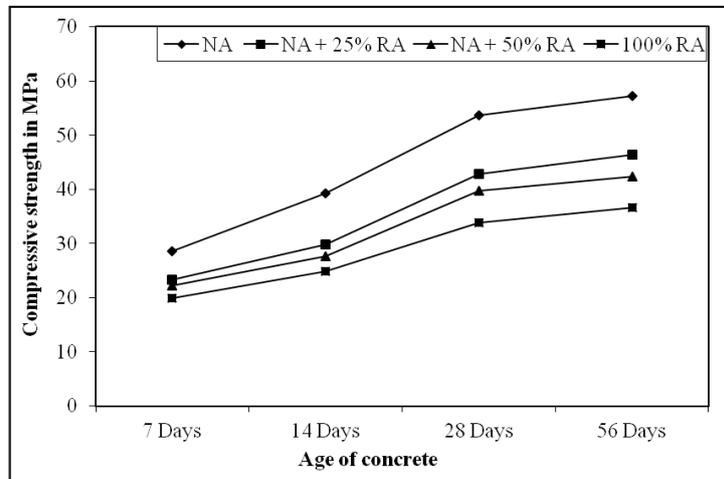
Fig. 1 Effect of RA on compressive strength
