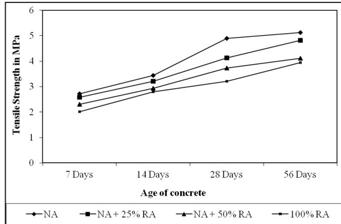
Fig. 3 Effect of RA on tensile strength
