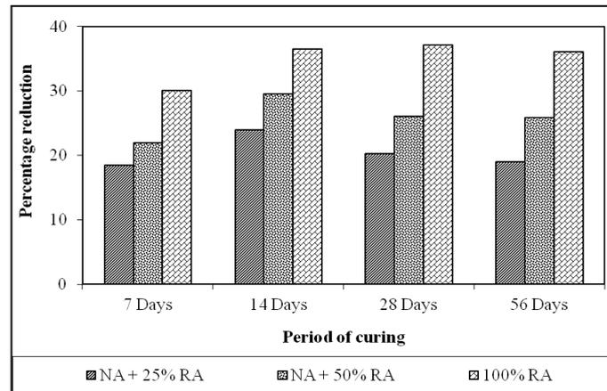
Fig. 2 Percentage reduction in compressive strength
