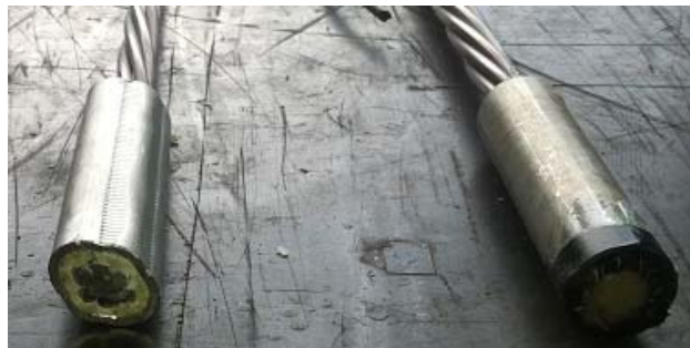
(a) Epoxy-filled aluminum tube
