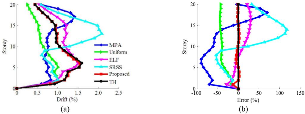
Fig. 4 (a) Drift profiles, (b) Drift errors, of all considered procedures due to Imperial Valley Array #6 earthquake record
