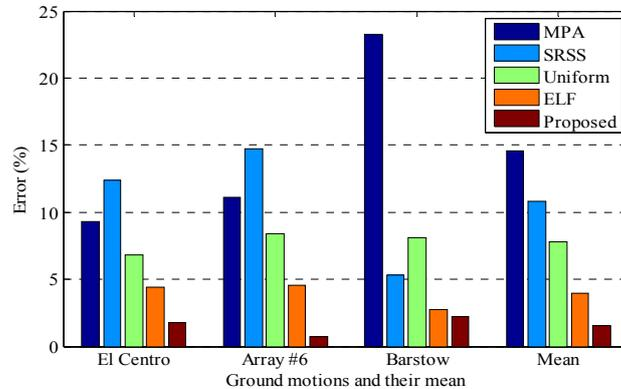
Fig. 6 Drift error for each NSP and each earthquake records and their mean value
