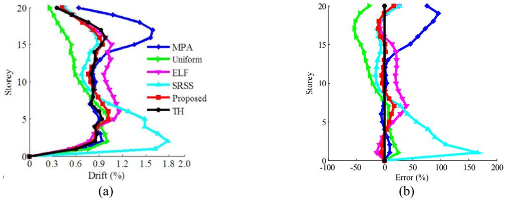
Fig. 3 (a) Drift profiles, (b) Drift errors, of all considered procedures due to El Centro earthquake record
