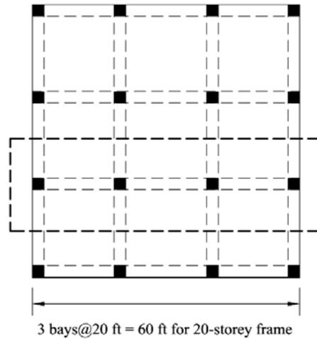
Fig. 2 Floor plan of the RC space moment frame building (1ft =0.30m)
