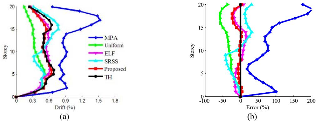
Fig. 5 (a) Drift profiles, (b) Drift errors, of all considered procedures due to Barstow earthquake record
