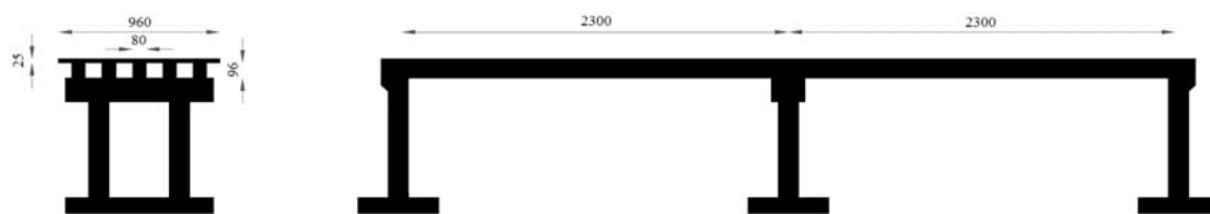
Fig. 2(b) Schematic views of two-span concrete highway bridge (Dimensions in cm)
