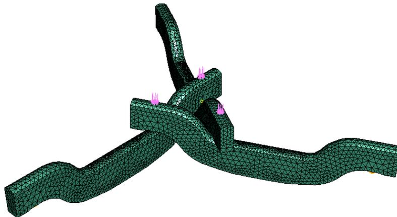
Fig. 4 Numerical model perspective view.  $P$  forces representing additional load are located over the reciprocal bearing points (see Fig. 3)
