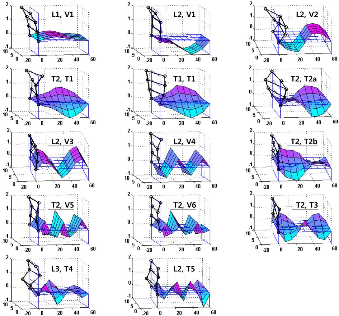
Fig. 9 Identified Mode shapes from the backward AR (RD) methods
