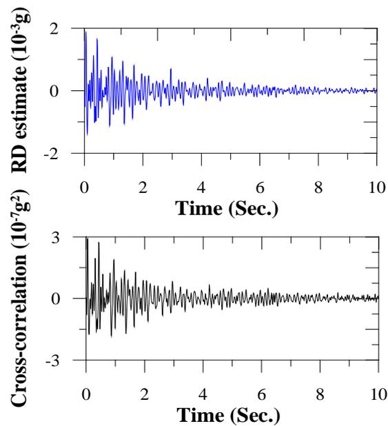
Fig. 7 RD estimate and cross-correlation function of an acceleration time series
