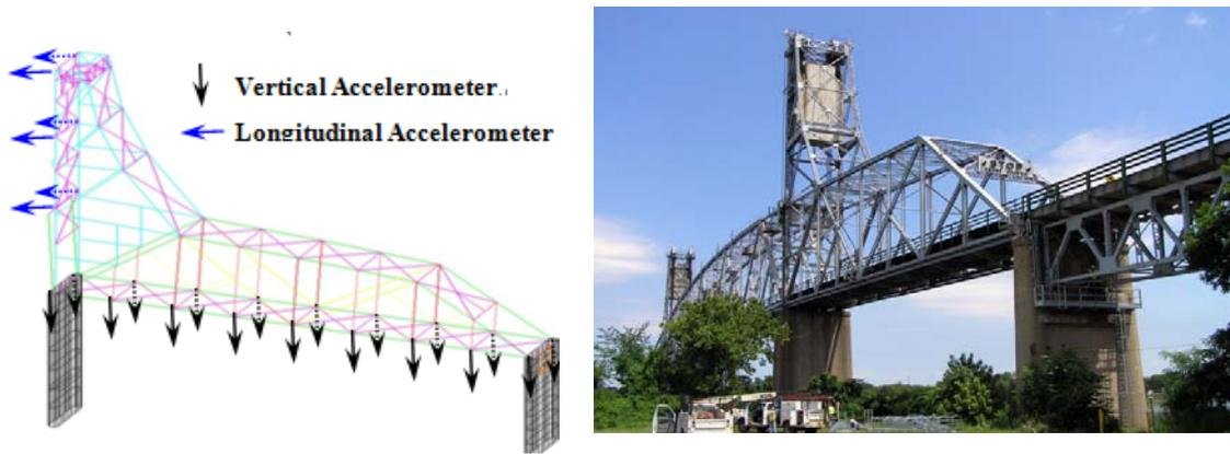
(a) Sensor layout on the tower span
