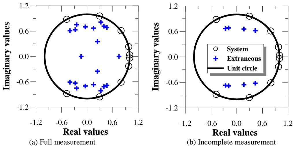
Fig. 4 Locations of the system and extraneous roots from the backward AR models
