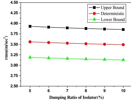
Fig. 13 The variation of the top floor rmsa with varying damping ratio of the isolator
