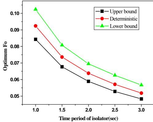
Fig. 10 The variation of the isolator normalized yield strength with varying time period of the isolator
