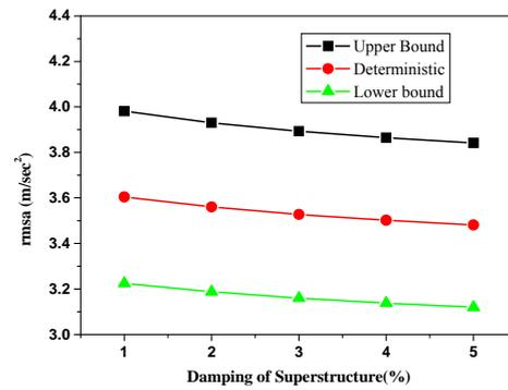
Fig. 7 The variation of the top floor rmsa with varying damping ratio of the superstructure
