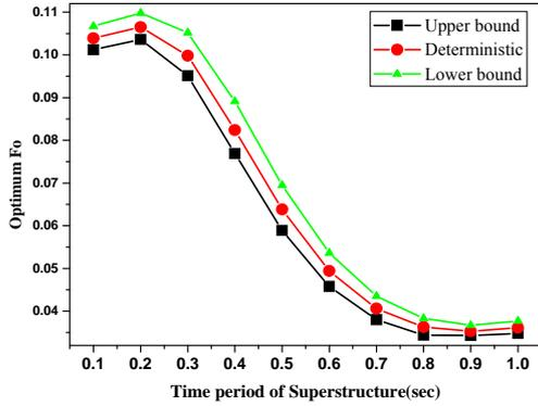
Fig. 4 The variation of isolator normalised yield strength with time period of the superstructure
