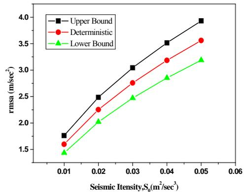
Fig. 9 The variation of the top floor rmsa with varying level of seismic intensity
