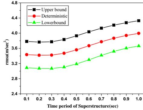
Fig. 5 The variation of the top floor rmsa with time period of the superstructure
