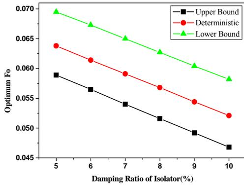
Fig. 12 The variation of the isolator normalized yield strength with varying damping ratio of the isolator
