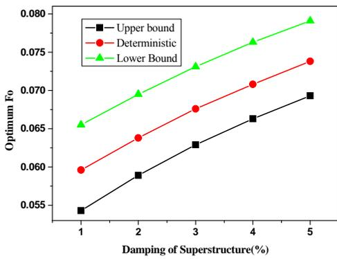
Fig. 6 The variation of isolator normalised yield strength with varying damping ratio of the superstructure
