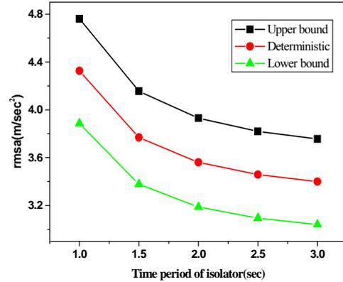
Fig. 11 The variation of the top floor rmsa with varying time period of the isolator
