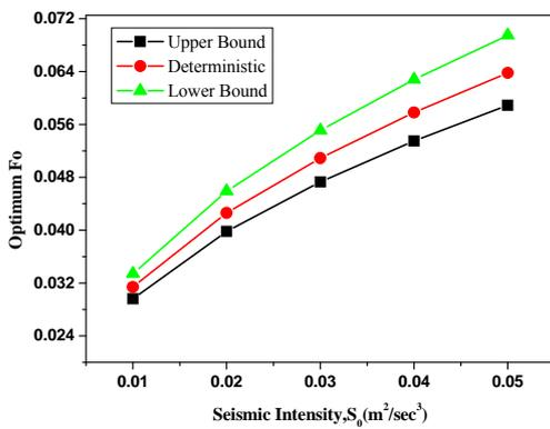
Fig. 8 The variation of isolator normalised yield strength with varying level of seismic intensity
