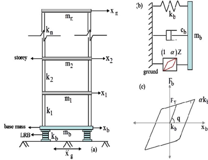
Fig. 1 (a) The idealized building frame with LRB (b) Idealization of the LRB isolator and (c) The bi-linear hysteretic model of the isolator
