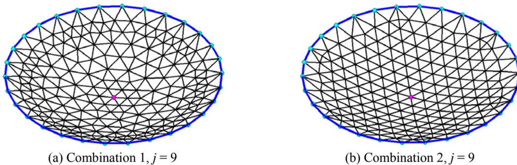
Fig. 9 Mesh configurations different from Fig. 7 by modifying boundary connection conditions
