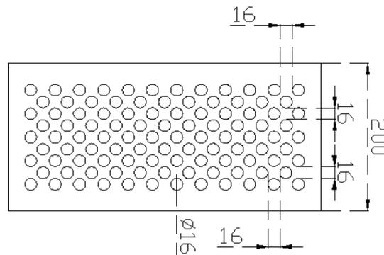
Fig. 1 Plate perforation pattern
