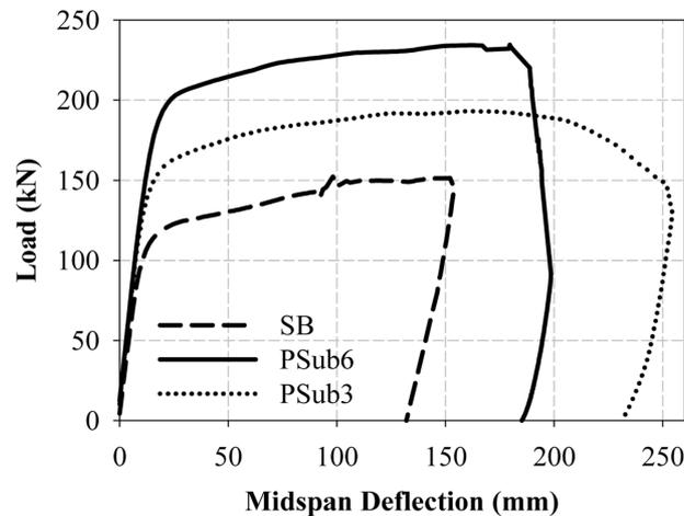
Fig. 7 Effect of plate thickness on flexural behavior
