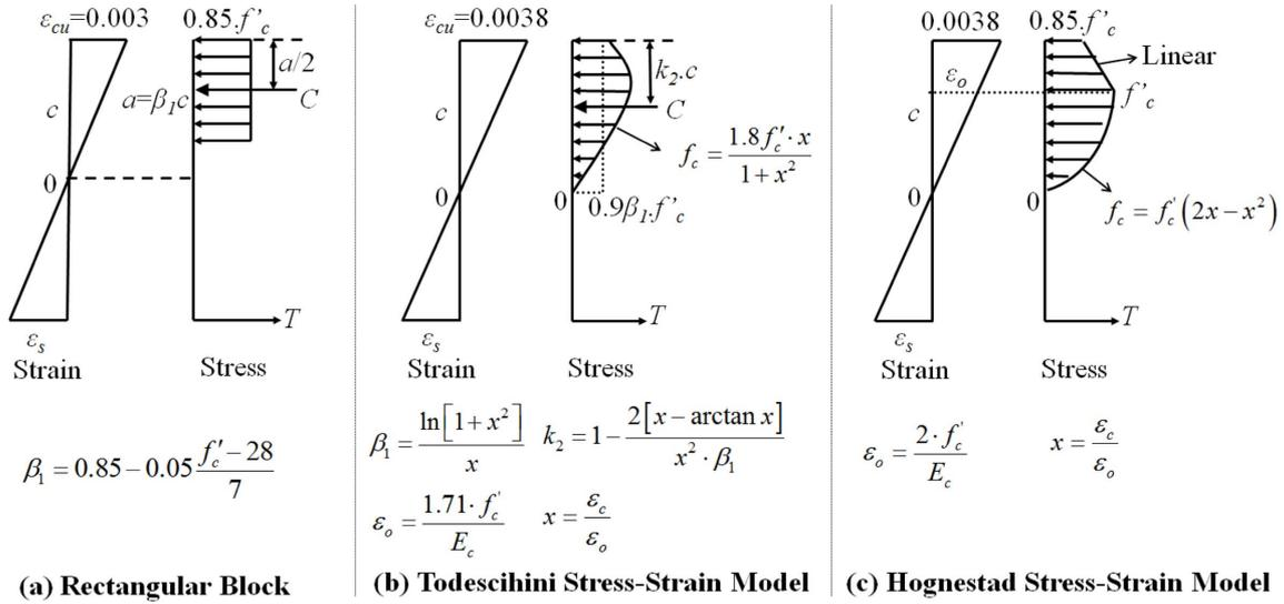
Fig. 5 Concrete stress-strain models used in ultimate load calculations
