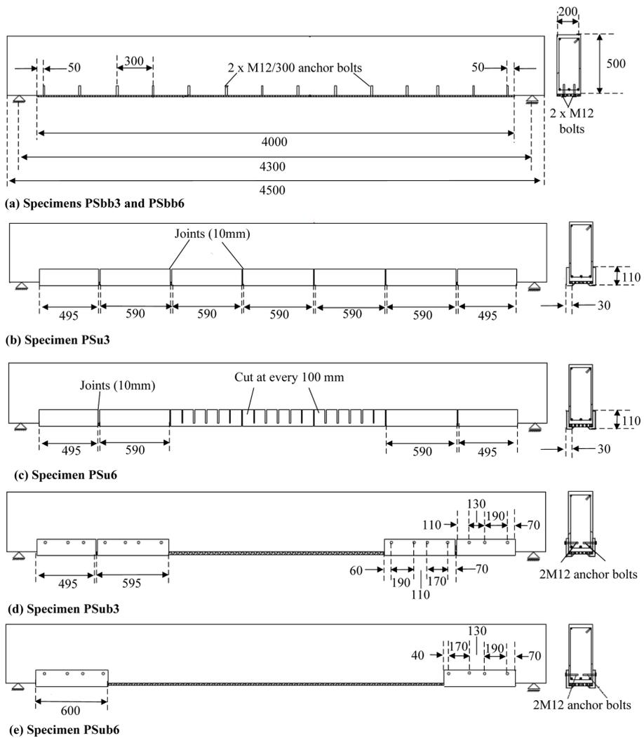
Fig. 3 Specimen details
