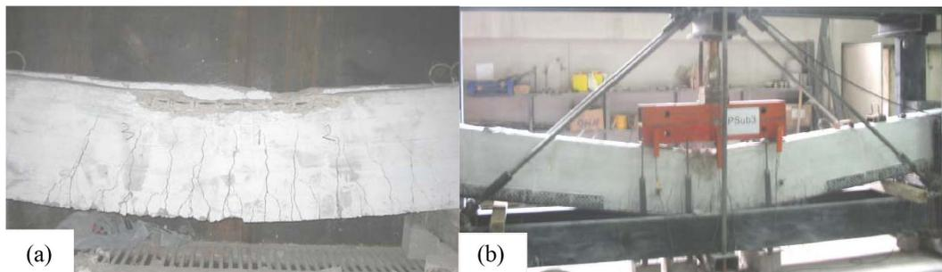
Fig. 4 Flexural failure of specimen (a) PSb3 (b) PSub3
