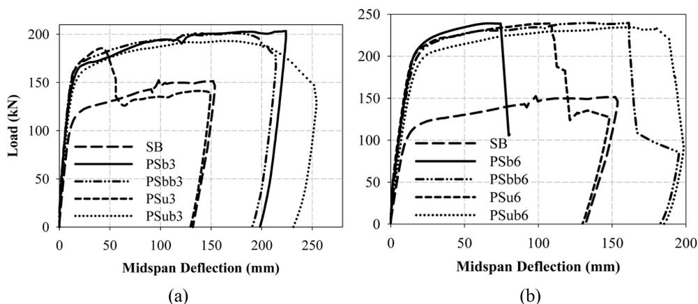
Fig. 6 Load-deflection curves of beams with (a) 3 mm (b) 6 mm external plates
