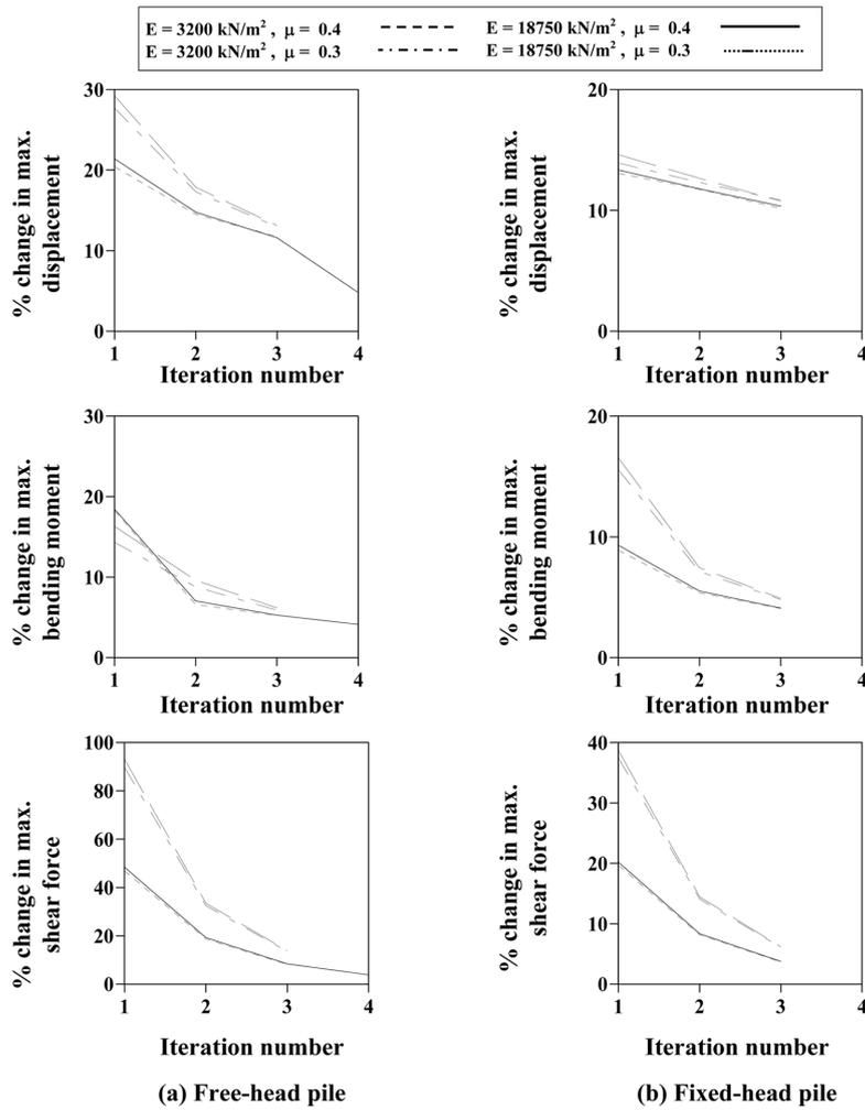
Fig. 2 Variation of change of response with respect to previous iteration
