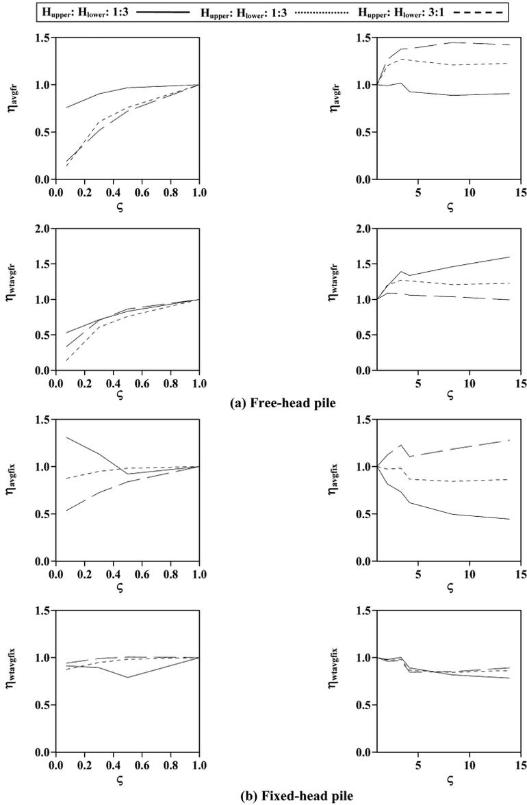
Fig. 8 Correction factors to determine the equivalent Young's Modulus of bi-layer soil for lateral capacity of pile
