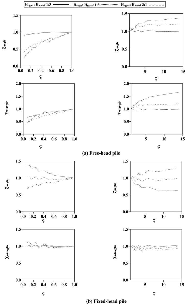
Fig. 7 Correction factors to determine the equivalent lateral capacity of pile in bi-layer soil
