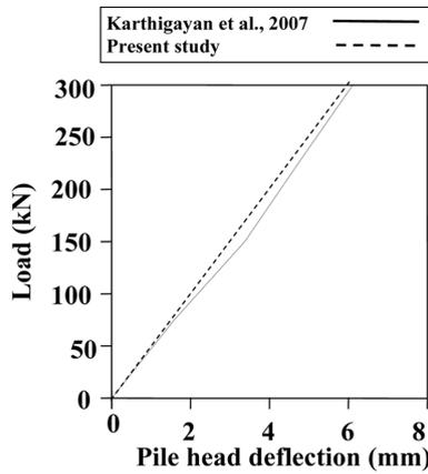
Fig. 5 Comparison of lateral load and pile head deflection with a previous study (Karthigayan *et al.* 2007)
