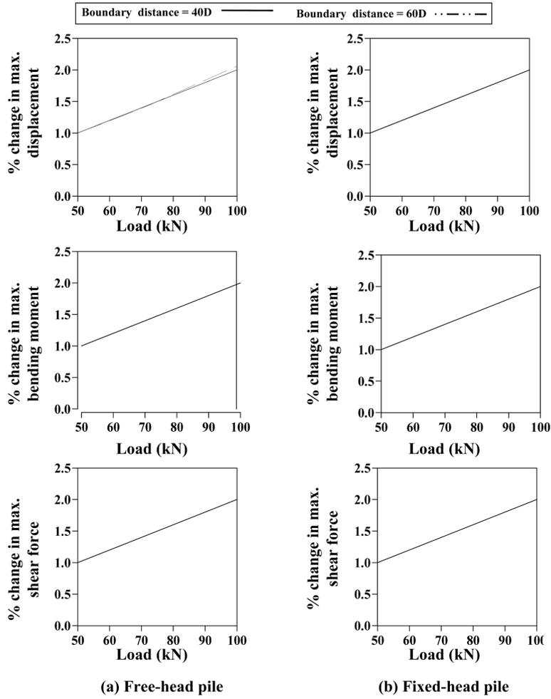
Fig. 4 Variation of normalized maximum response with increase of lateral load
