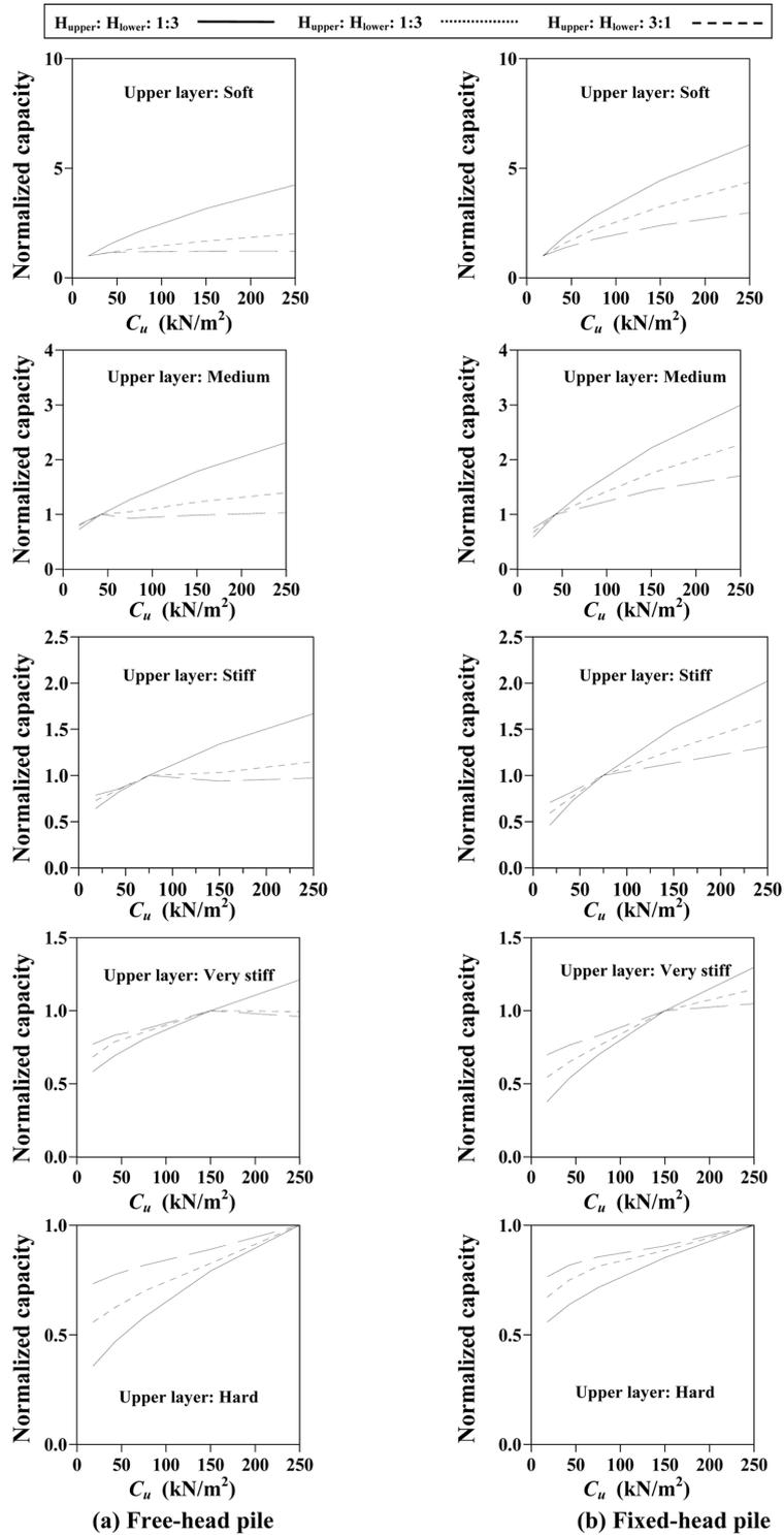
Fig. 6 Variation of lateral capacity in bi-layer media normalized to capacity in homogeneous soil conforming to upper layer
