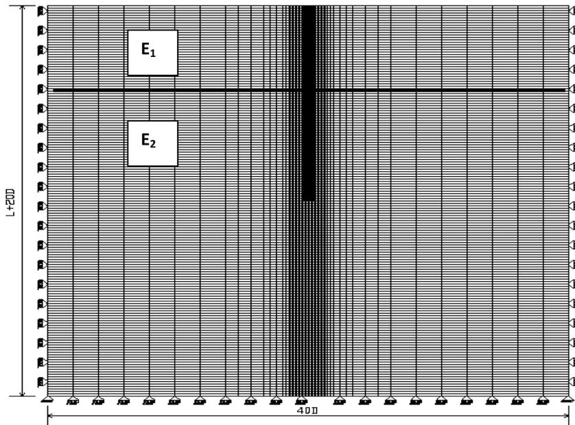
Fig. 1 Schematic representation of soil-pile system discretized in the mathematical model
