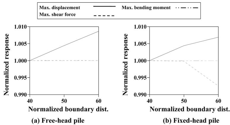
Fig. 3 Variation of normalized maximum response with increase of distance of the boundary
