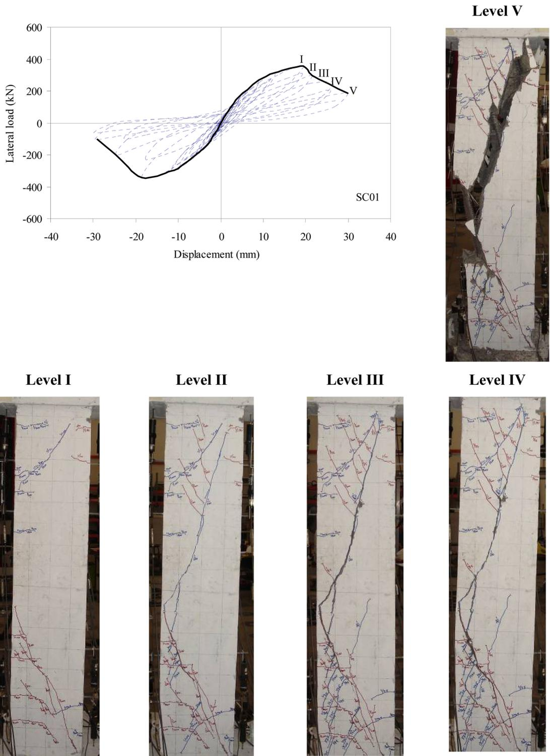
Fig. 7 Cracking patterns of tested specimen
