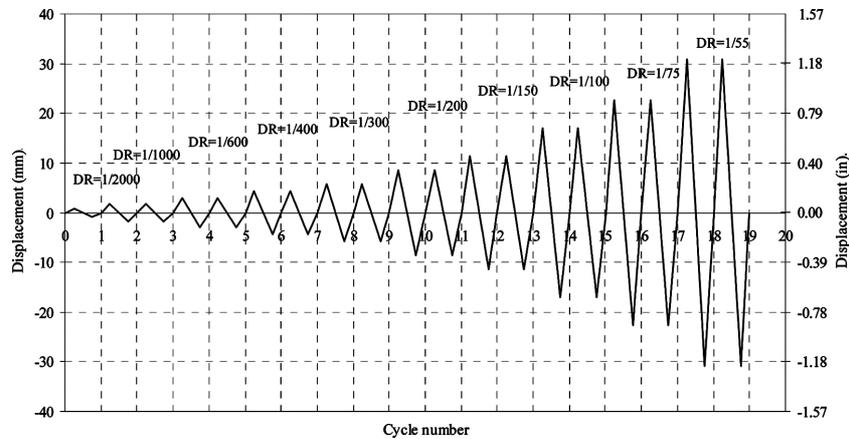
Fig. 5 Loading procedure
