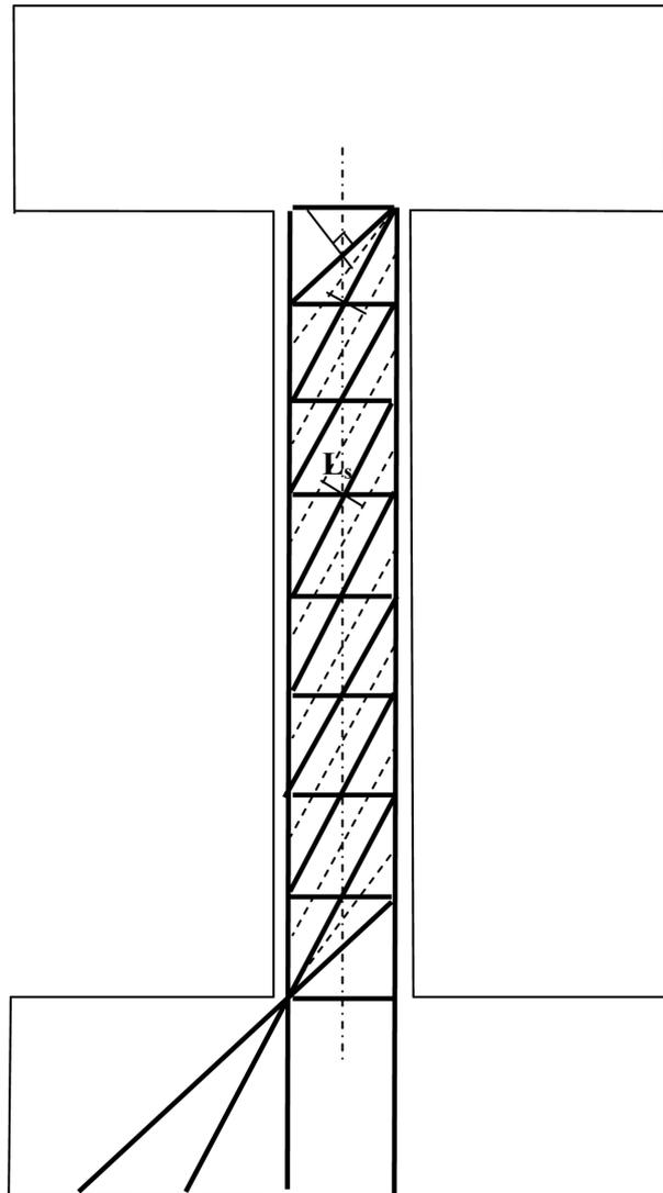
Fig. 2 Sizing of inclination struts
