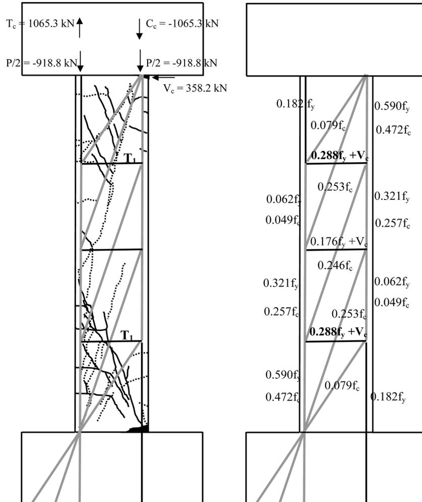
Fig. 8 Resisting mechanism at the ultimate shear capacity
