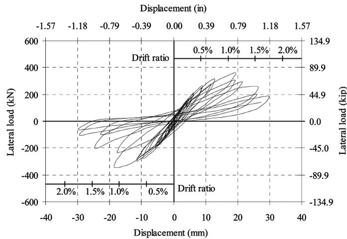
Fig. 6 Hysteresis loops of specimen SC01
