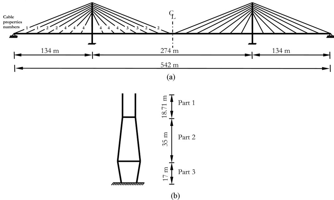
Fig. 2 Details of (a) the cable-stayed bridge model, and of (b) the towers
