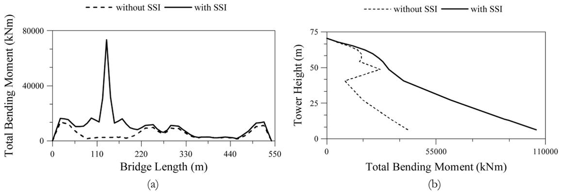
Fig. 12 Total bending moment of the bridge founded on soft soil; (a) deck, (b) tower
