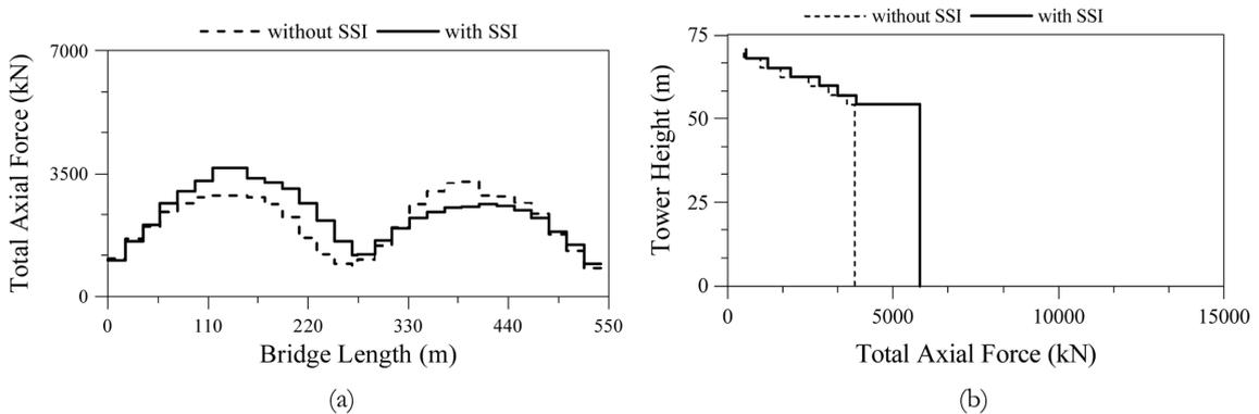
Fig. 7 Total axial forces of the bridge founded on medium soil; (a) deck, (b) tower
