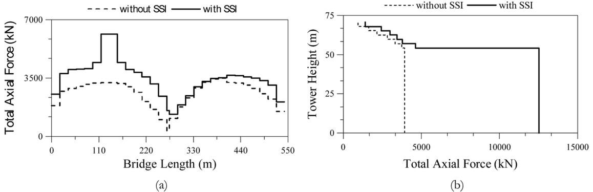
Fig. 6 Total axial forces of the bridge founded on soft soil; (a) deck, (b) tower
