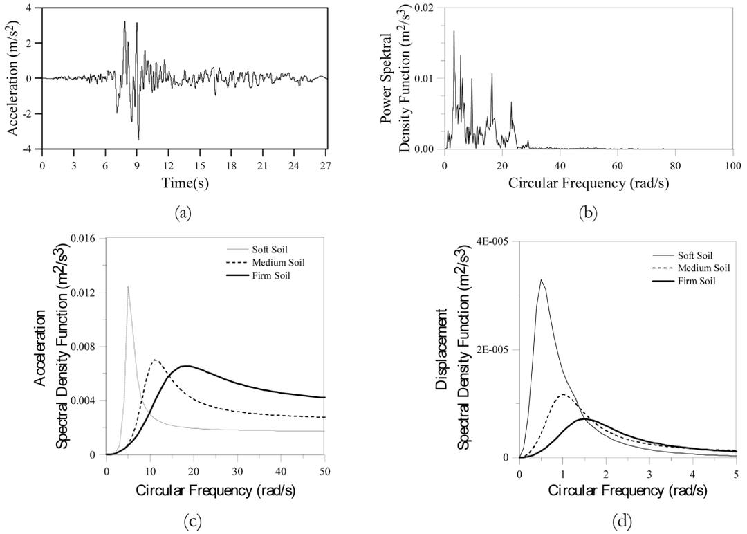
Fig. 3 The DZC270 component of the 1999 Kocaeli, Turkey, earthquake; (a) acceleration time history, (b) power spectral density function, (c) acceleration spectral density function, (d) displacement spectral density function
