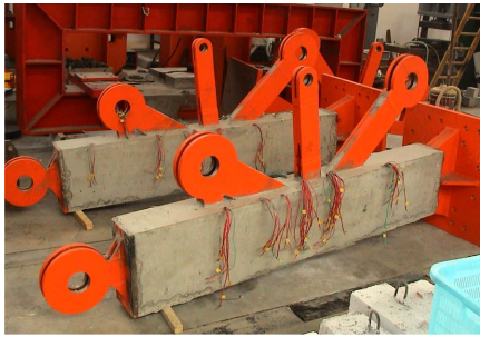
Fig. 8 Joint made of steel-concrete
