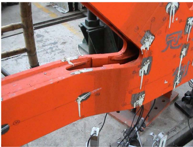
Fig. 10 Failure pattern of joint made of steel
