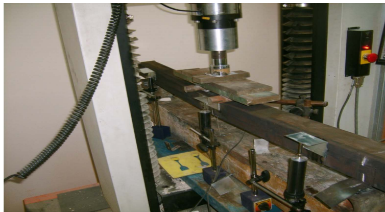
Fig. 3 The view of the BF3-1 under four-point bending at the test time
