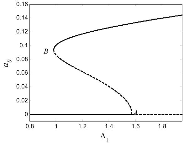
Fig. 8 Variations of  $a_0$  with respect to the variations of  $\Lambda_1$  for system with  $\alpha_2 v_p^2 = 35$ ,  $\sigma = 0.05$ . Solid lines belong to stable solution, and dashed lines belong to unstable solution
