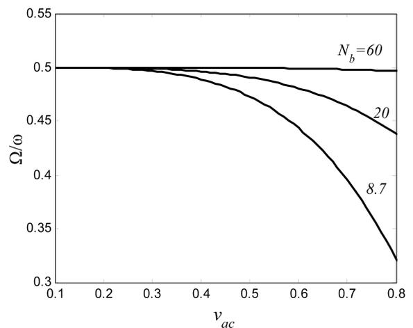
Fig. 10 Variations of  $\Omega/\omega$  with respect to the variations of  $v_{ac}$  for different values of  $N_b$ , where  $\alpha_2 v_p^2 = 60$
