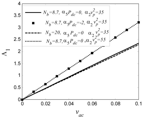
Fig. 3 Variations of  $\Lambda_1$  with respect to the variations of  $v_{ac}$  for different values of system parameters, where,  $\alpha_2 = 2.95, h_p/h_b = 0.1, v_{ac} = 0.02, \mu = 0.04, l_2 - l_1 = 0.4l$
