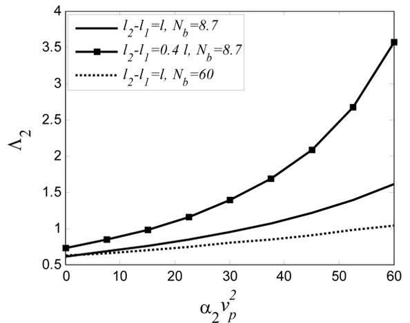
Fig. 4 Variations of  $\Lambda_2$  with respect to the variations of  $\alpha_2 v_p^2$  for different values of system parameters, where  $v_{ac} = 0.5, h_p/h_b = 0.1, \mu = 0.04, \alpha_2 = 2.95, \alpha_5 P_{dc} = -2$
