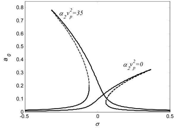
Fig. 12 Variations of  $a_0$  with respect to the variations of  $\sigma$  for different values of  $\alpha_2 v_p^2$  where  $v_{ac} = 0.2$ . Solid lines belong to stable solution, and dashed lines belong to unstable solution
