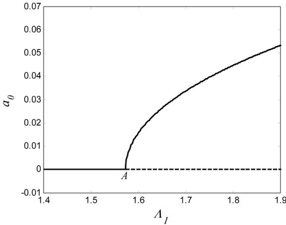
Fig. 7 Variations of  $a_0$  with respect to the variations of  $\Lambda_1$  for the system with  $\alpha_2 v_p^2 = 35$  and  $\sigma = -0.05$ . Solid lines belong to stable solution, and dashed lines belong to unstable solution
