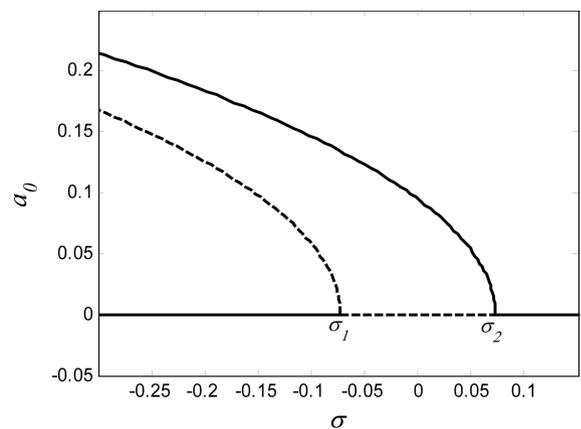
Fig. 6 Variations of  $a_0$  with respect to the variations of  $\sigma$  for the system with  $\alpha_2 v_p^2 = 55$ ,  $v_{ac} = 0.06$ ,  $S < 0$  Solid lines belong to stable solution, and dashed lines belong to unstable solution
