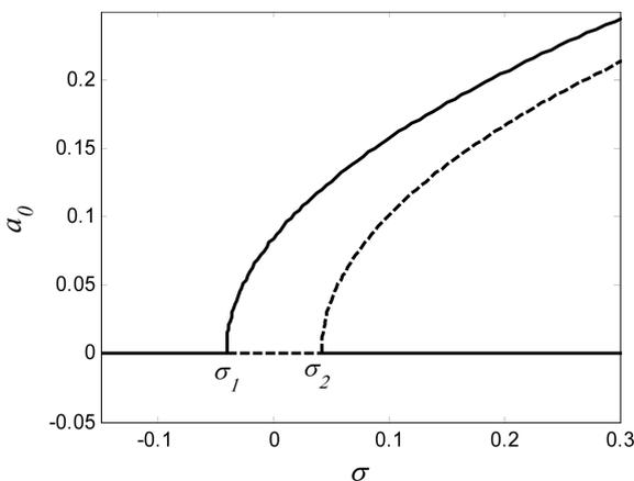
Fig. 5 Variations of  $a_0$  with respect to the variations of  $\sigma$  for system with  $\alpha_2 v_p^2 = 35$ ,  $v_{ac} = 0.06$ ,  $S > 0$ . Solid lines belong to stable solution, and dashed lines belong to unstable solution
