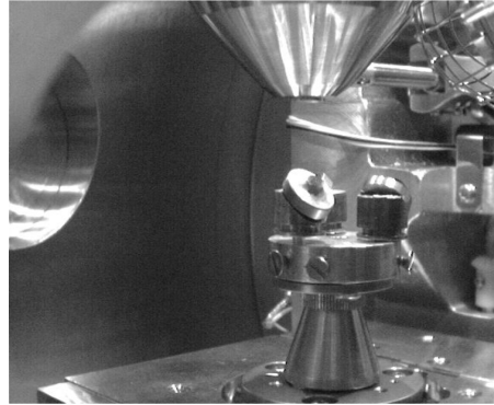
Fig. 11 Scanning electron microscope set-up
