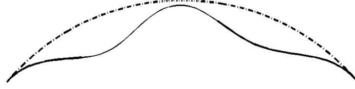
(a) The third mode shape, \phi_T=100^\circ, f_3=1826.09 Hz
