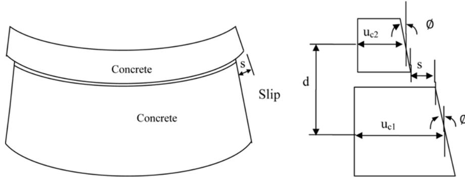
Fig. 3 Partial composite action
