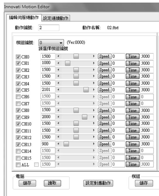
Fig. 6 Number in Motion Editor when the robot stands up slowly
