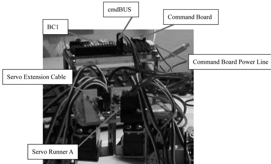
Fig. 2 The upper part is controlling panel area
