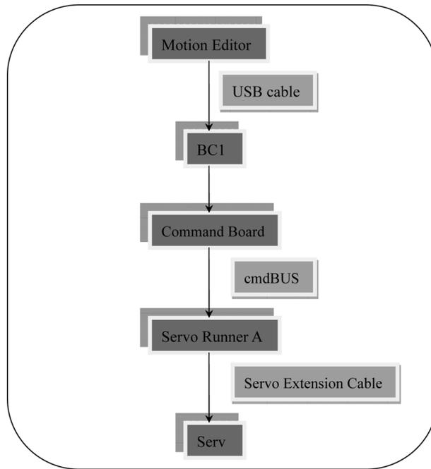
Fig. 4 This is flow chart which the program performs the movements on 12-DOF Bipedinno robot
